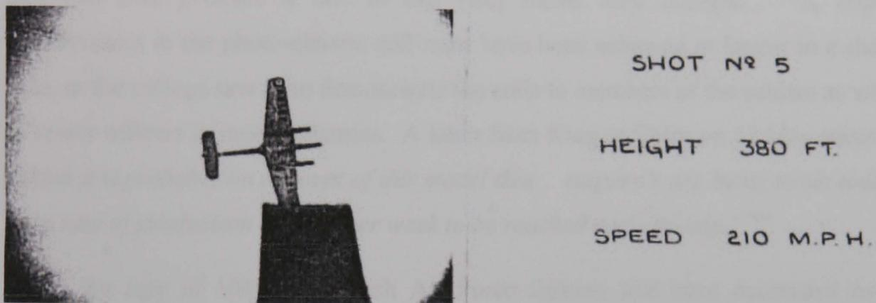
Fig. 7.14 A trial recorded in AVIA 13/874 on the 14<sup>th</sup> of March 1939 of the photo-electric cell mounted in the nose of a Bristol Blenheim aircraft, serial L.1254. The aircraft being detected has the distinct outline of an Armstrong-Whitworth Whitley, although this type is not mentioned in the file.
