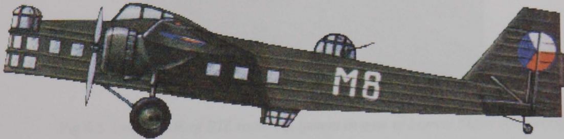
Fig. 6.4 Marcel Bloch 200 aircraft. Unlike the aircraft used by BTL, this aircraft has Czechoslovakian national markings and is fitted with a dorsal and ventral turret.
