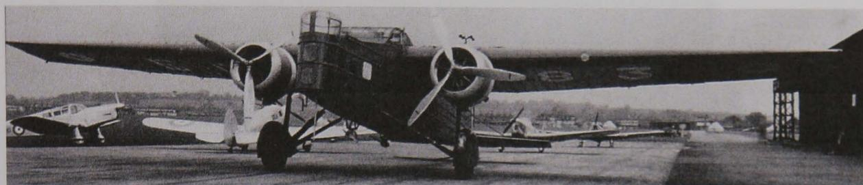
Fig. 6.8 *The MB 200 at Hendon aerodrome. Note the absence of the ventral turret and single bladed generator fitted below fuselage.*
