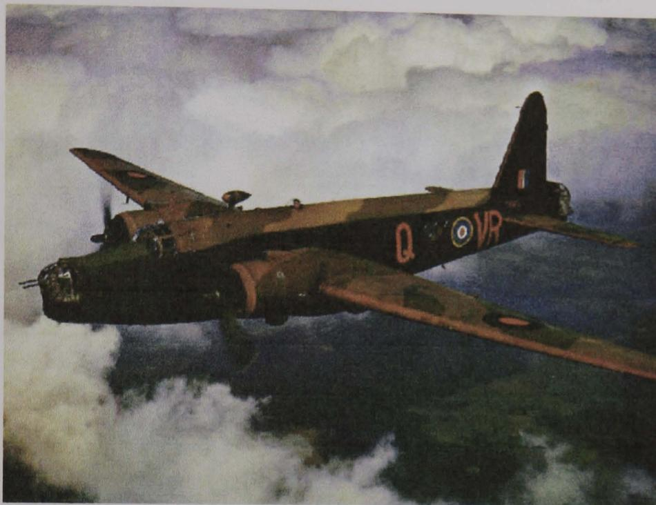
Fig. 6.24 A Vickers Wellington Mk 1C aircraft
