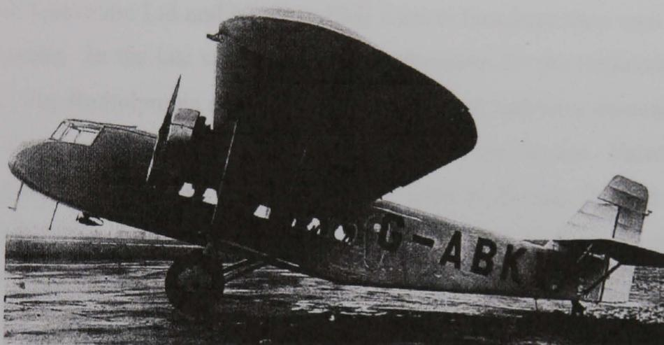
Fig. 6.11 *The Blackburn CA.15.C. experimental aircraft which was fitted with Marconi-EMI television equipment in 1936*
