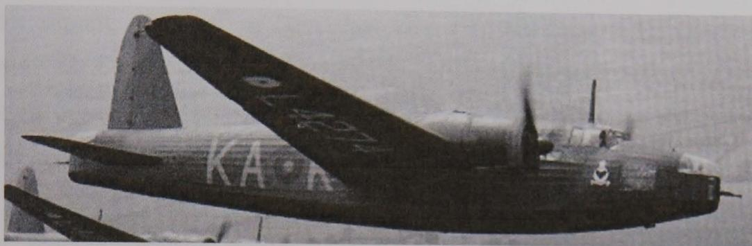
Fig. 6.26 *Wellington Mk I fitted with Vickers Turrets*
