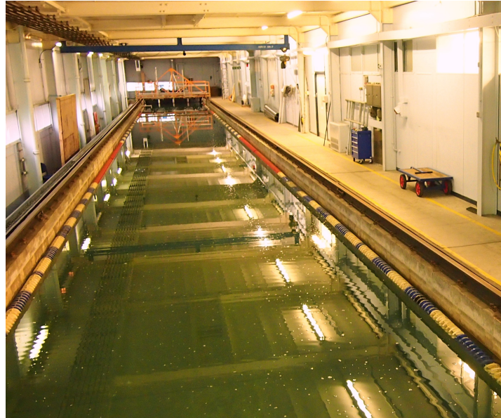
Figure 3.6: Photograph along the length of the Kelvin Hydrodynamics Laboratory's tow tank, taken from the tow carriage during testing in 2013
