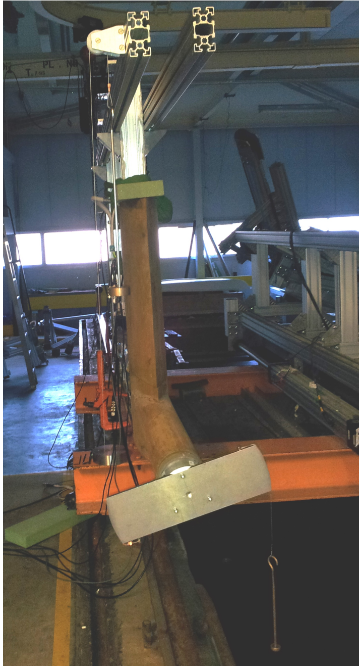
Figure 3.13: Calibration of torque transducer using mass weights and a pulley system, equal force was applied to each side of the hub for accurate torque calibration.
