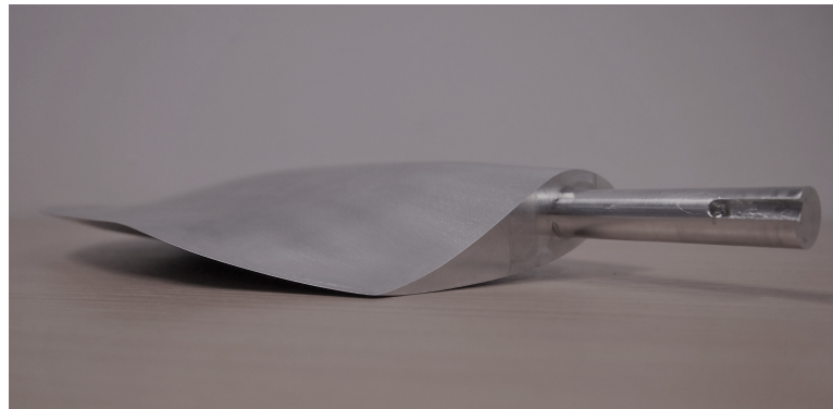
Figure 5.13: Photograph of a blade before testing. Slot for pin can be seen on blade root shaft, as well as the twist distribution and the root aerofoil section.
