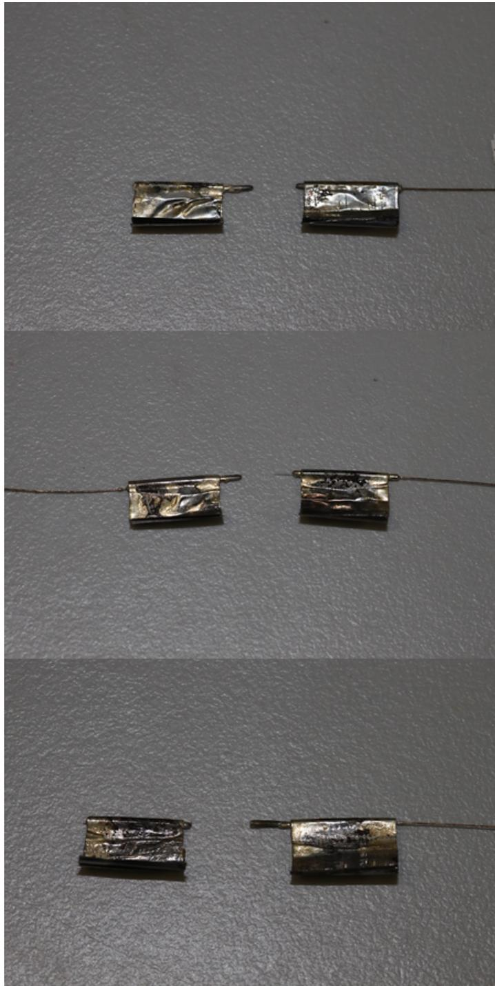
Fig. 5.12 Three FBG strain sensors tested to failure; each time the capillary broke first demonstrating that the brazed joints between the shim and capillary are of adequate strength.
