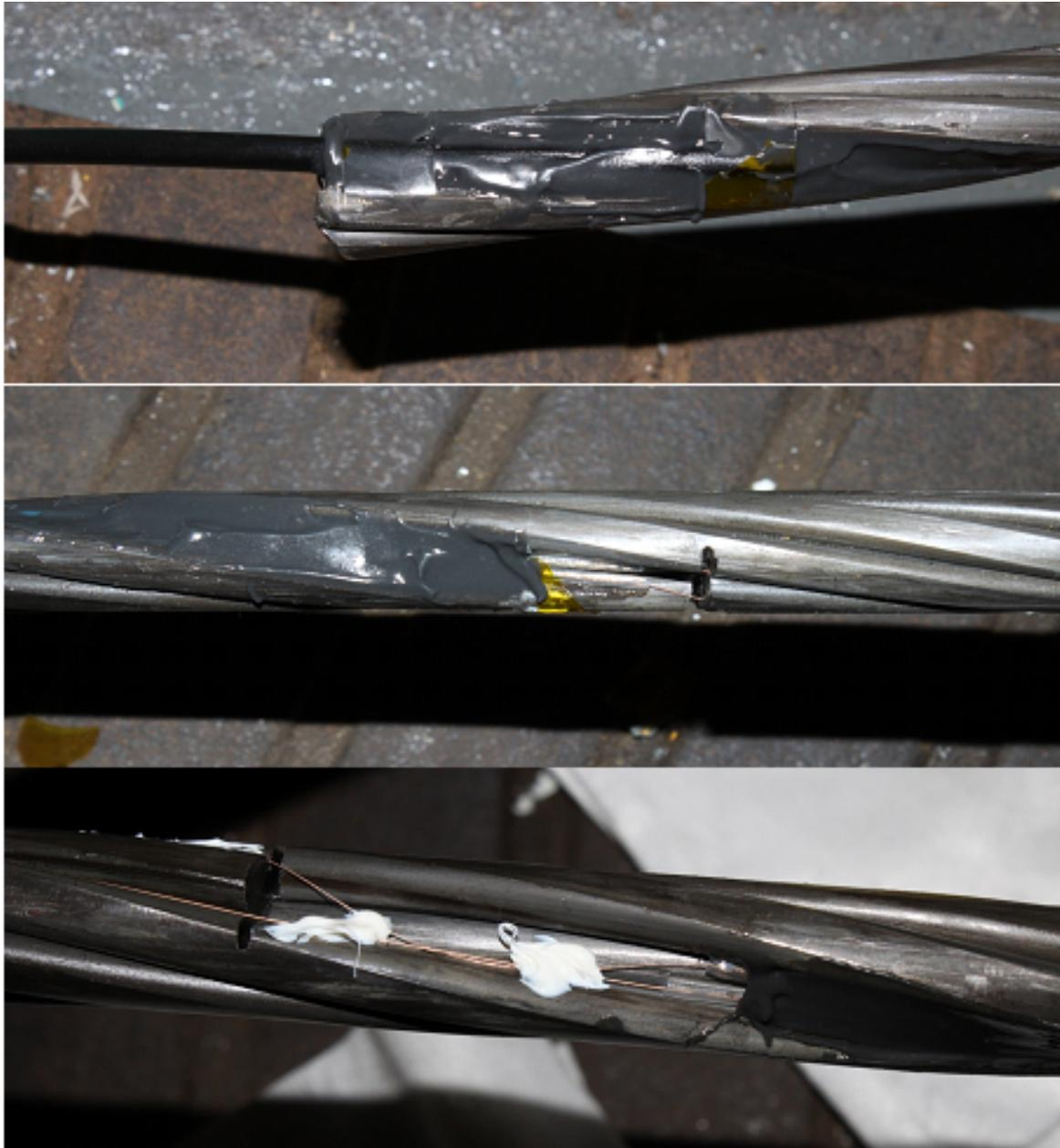
Fig. 7.5 Photos of the cut outer wire and reinforced fibre cable exiting the strand. Epoxy covers the splice protectors and fibre cable holding them in place.
