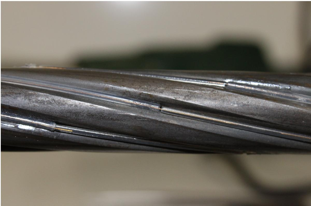
Fig. 5.16 The interrogating fibre was inserted into silicone tubing to prevent it coming out of the groove if the strand was bent.
