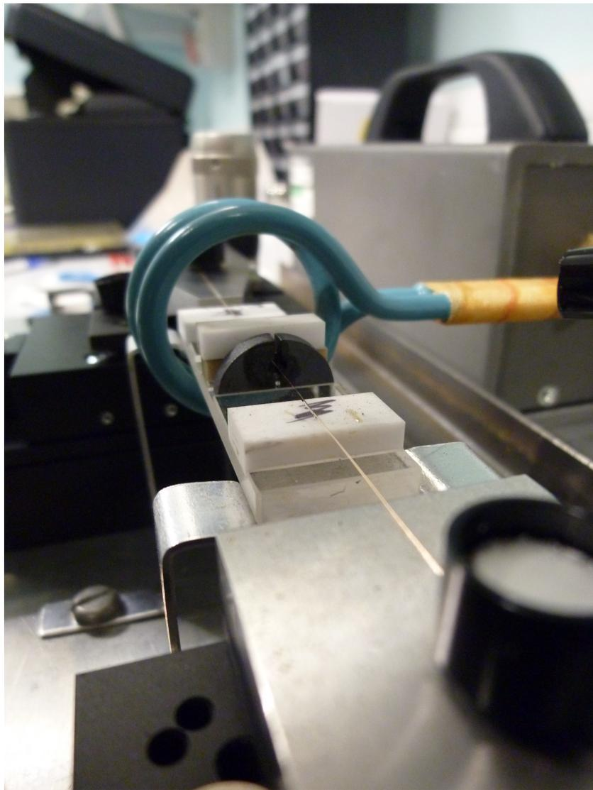
Fig. 5.2 The induction heating rig. An alternating current flows through the coil, heating the ferromagnetic material within.
