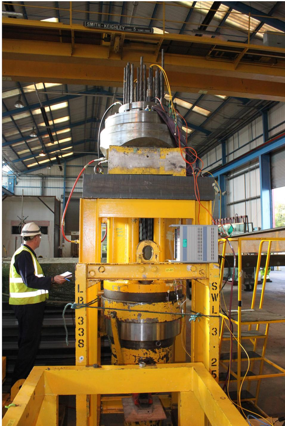
Fig. 8.1 28-strand calibration rig. The rig is used to calibrate a 28-strand stress jack, seen at the top, with a Statimeter load cell.
