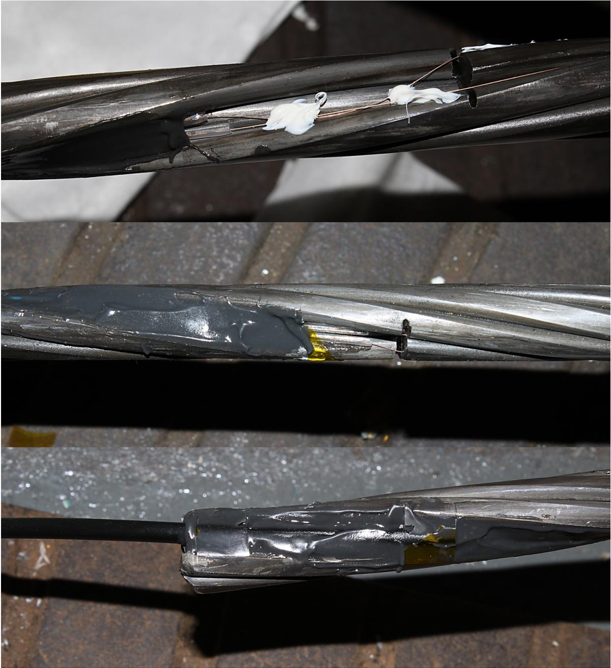
Fig. 5.19 Photos of the cut outer wire and reinforced fibre cable exiting the strand. Epoxy covers the splice protectors and fibre cable holding them in place.
