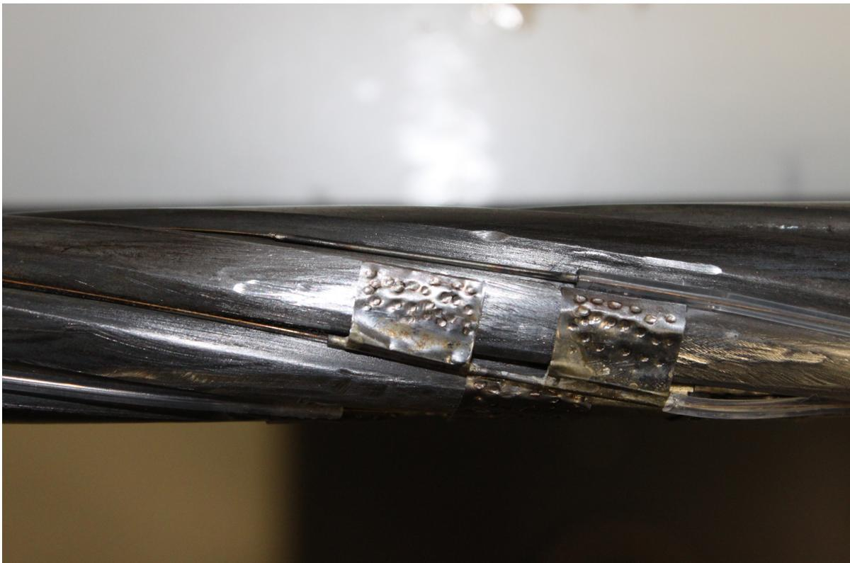
Fig. 5.14 When the temperature sensors were attached with silicone sealant at one end they showed some strain sensitivity. Consequently, for further tests, they were not attached to the strand but held in place by the interrogating fibre inside silicone tubing.
