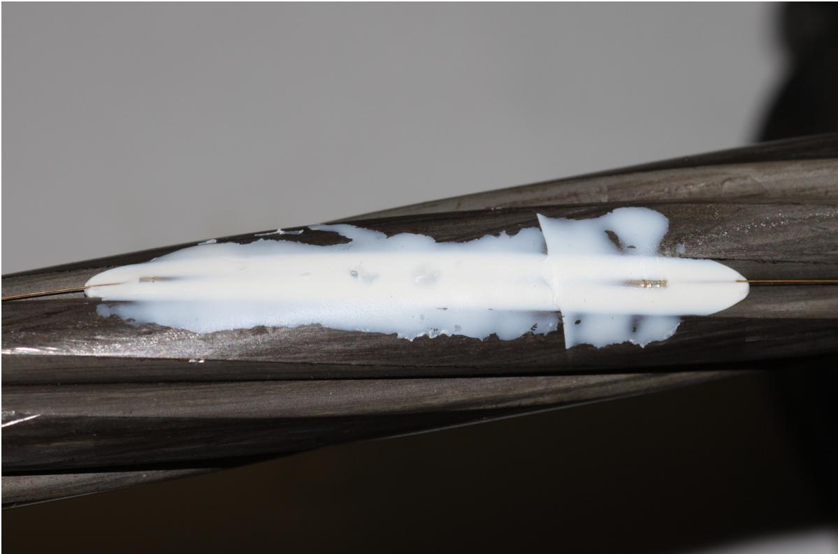
Fig. 5.15 Securing a splice protector to a prestressing strand with silicone sealant.
