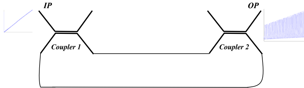
Fig. 4.14: Fiber ring resonator using two 3-dB couplers.
