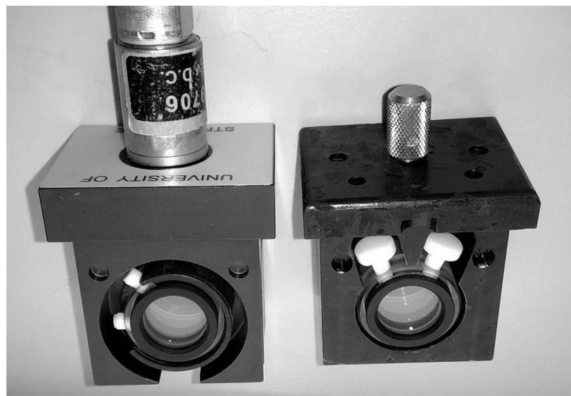
Figure 4-3 Photograph of the motorised rotating cell holder (left), developed at the University of Strathclyde and standard circular cell holder (right). Both are shown containing circular cells, the stoppers used for the rotating cell were modified to allow for free movement.
