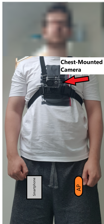
Figure 5.1 Photograph of recording setup for the data collection study (AP = ActivPAL).
