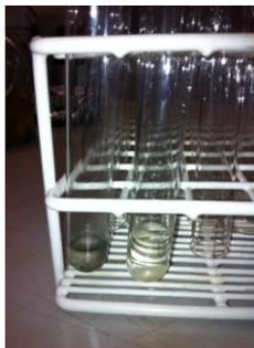
Figure 4.5: Acid group test, positive result (left) compared to negative result (right).
