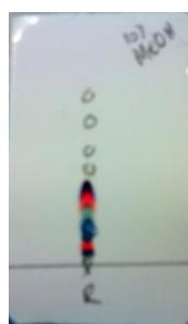
Figure 5.4: TLC of crude mixture from synthesis of dye 1, scheme 5.7, carried out in 9:1 DCM: MeOH
