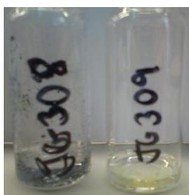
Figure 4.6 Ninhydrin test: free amine containing resin (left); and negative resin (right)
