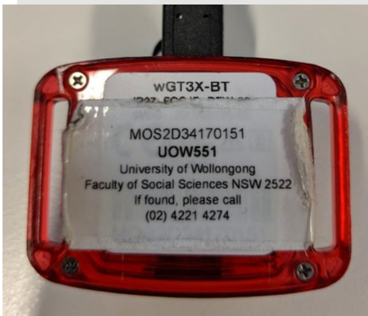
Figure 2: A GT3X+ accelerometer with an example of serial number label
