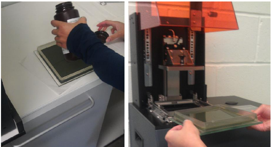
Fig. 32 showing the resin as it is being installed into the machine. From this pool of resin, the solid object will be synthesized using UV light. The object will emerge from the pool layer by layer.
