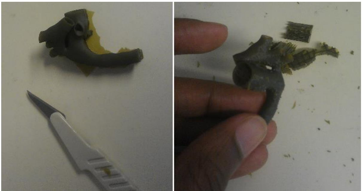
Fig. 25 showing the removal of the supports added prior to printing in order to provide the necessary reinforcement during synthesis. The removal of these supports leave the completed model behind.
