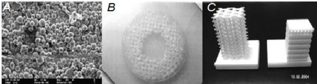
Fig 14. (A) showing the powder for SLS, (B) shows the sintered sample and (C) shows the nylon scaffold.
