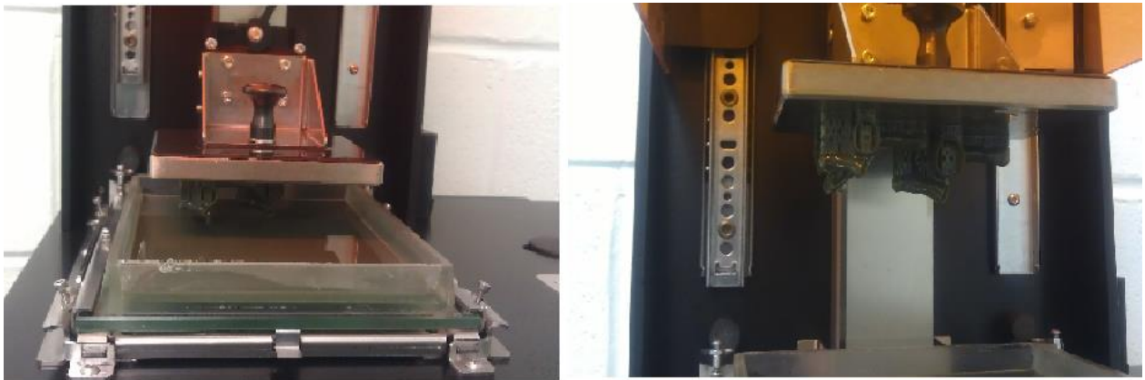
Fig 21. showing the models upon completion just as they are raised from the pool of resin.
