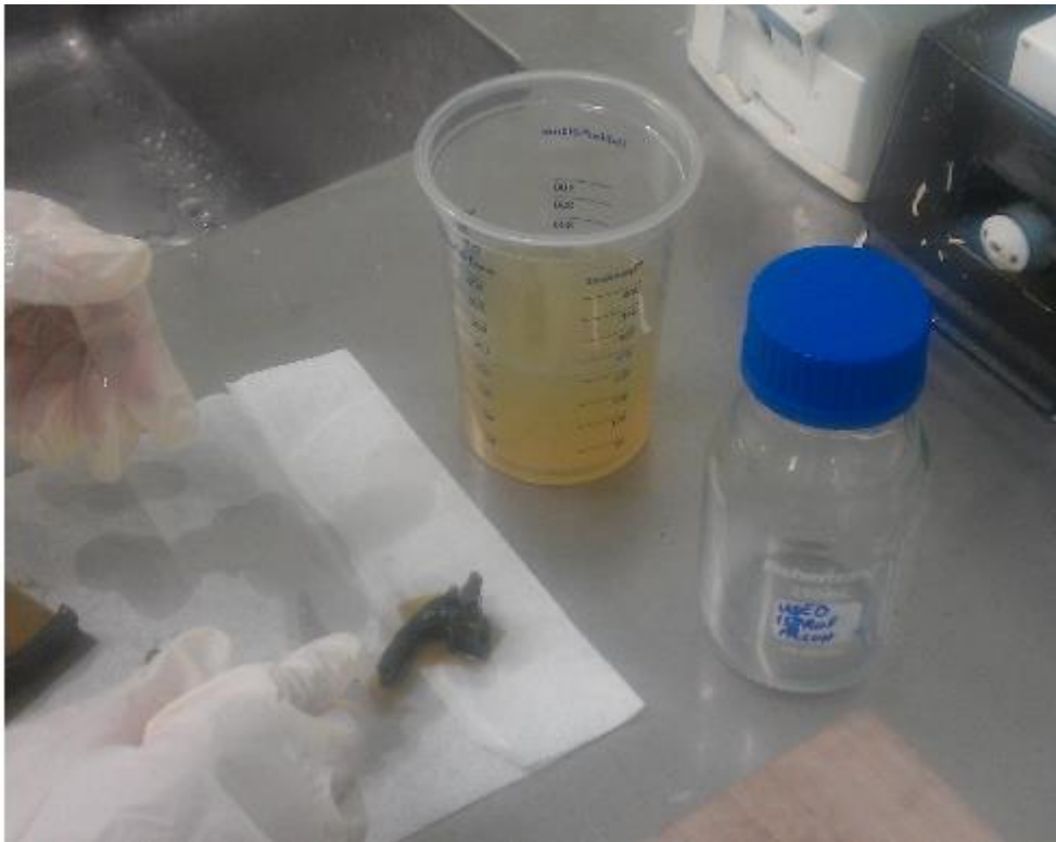
Fig 24. showing the models being washed in a bath of isopropanol and left to dry on a paper towel.
