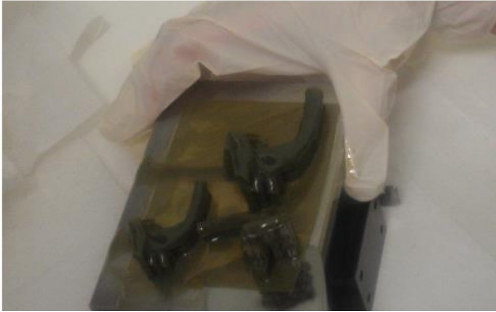
Fig 22. showing the models as they are being removed from the platform on which they were made. At this point the three models are connected by a thin layer of solidified resin on the platform.
