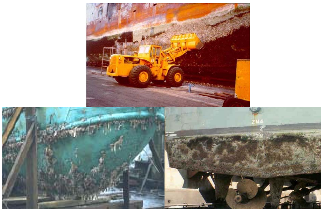
Figure 1.4 The fouling on ship hull (Yebra et al., 2004)
