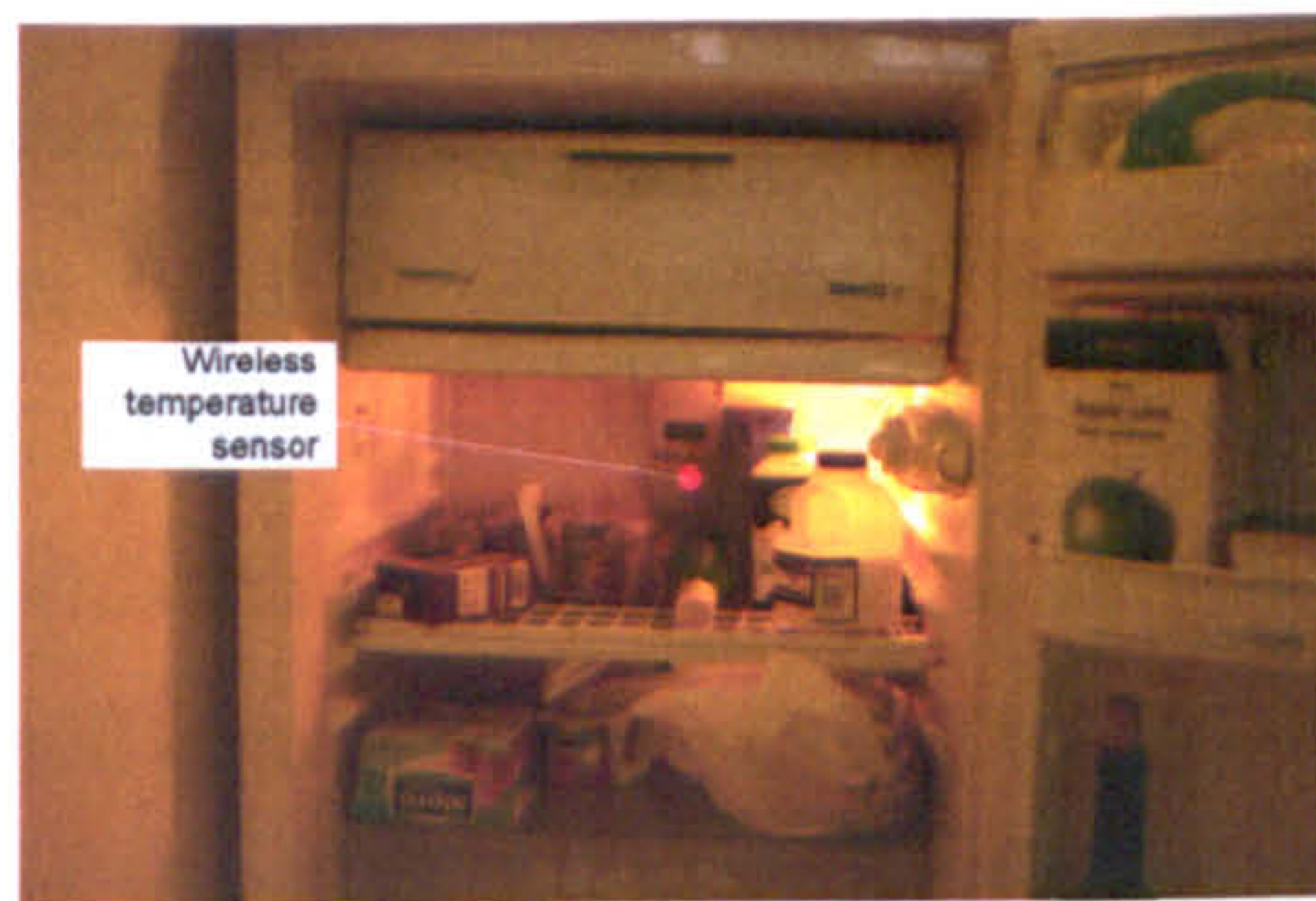
Wireless SMART temperature sensor inside refrigerator
