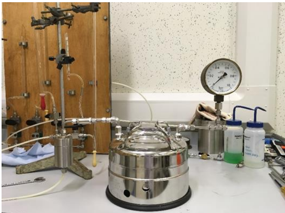
S.10 Gas and Pure water membrane test rig setup
