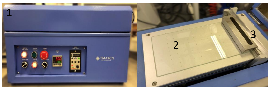
S.5 The casting machine setup for Flat sheet membranes preparation. 1. Casting machine 2. Glass plate 3. Casting knife
