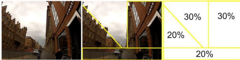
Figure 24 – Example of the proportion of sky ahead. Estimate of the proportion of sky ahead is approximately 30 per cent. (Location: Ingram St. 55°51'34.8"N 4°14'49.0"W)
