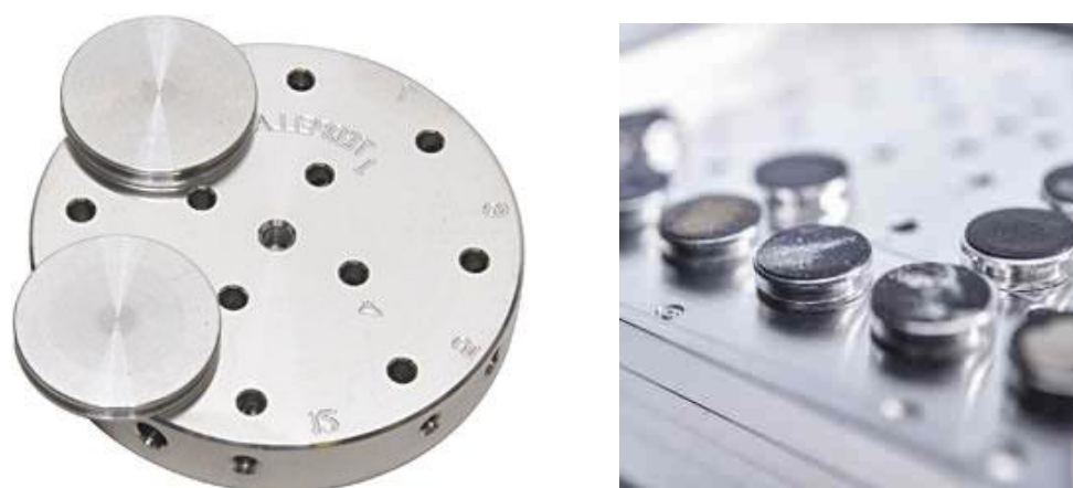
Figure B.1.1: Labeled image of the sample holder and sample wheel used for SEM analysis.
