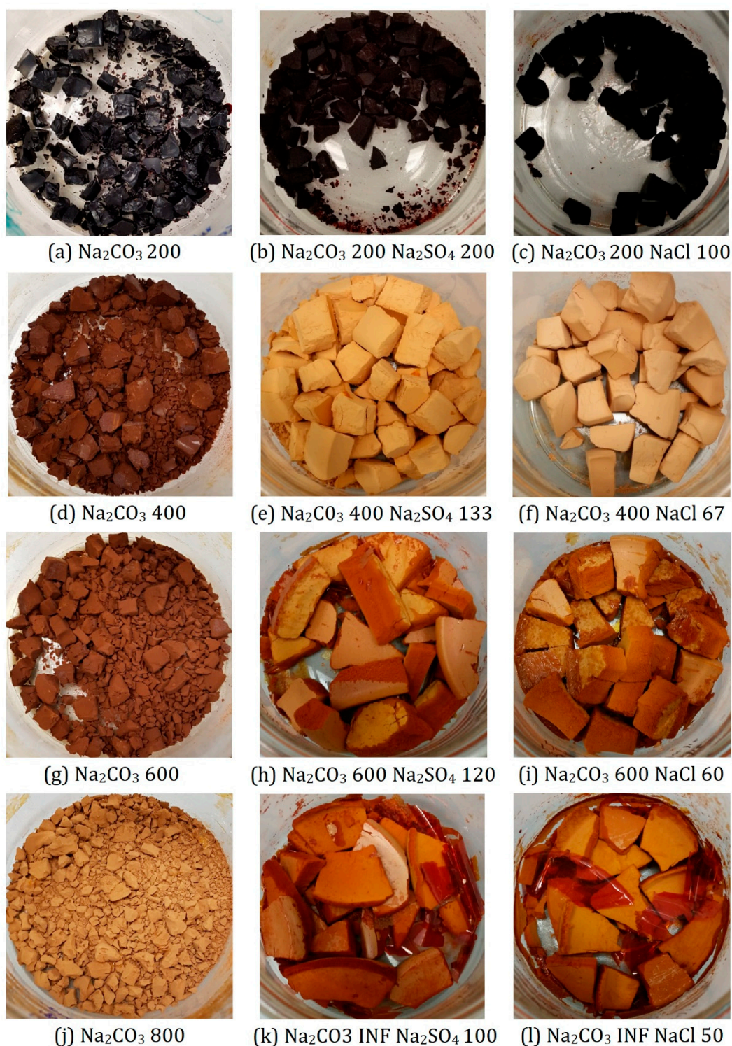
Figure 11. RF xerogels prepared with varying R/C ratios of \text{Na}_2\text{CO}_3 , \text{Na}_2\text{SO}_4 , and NaCl.
