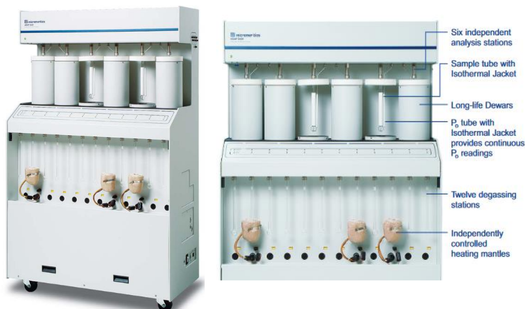
Figure 5.1: Labeled diagram of the Micromeritics ASAP 2420 Surface Area and Porosity Analyser used for nitrogen adsorption analysis.[221]
