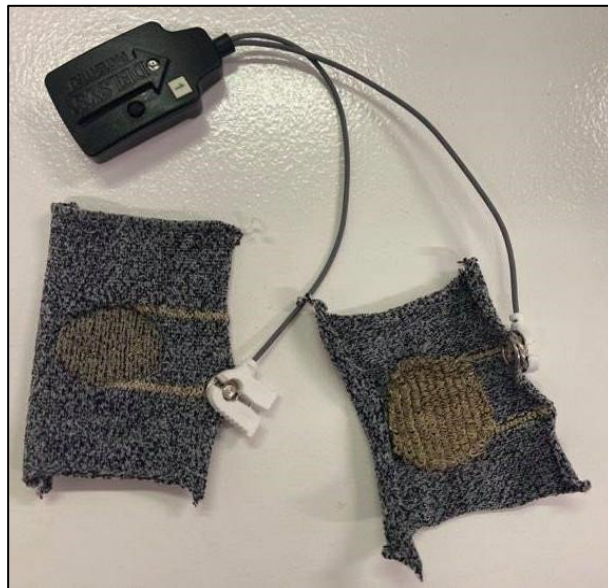
Figure 19 - Image of the Prototype 1 fabric base with copper stitched EMG electrode connected to a Delsys Trigno wireless unit as used in Stage 1 testing.
