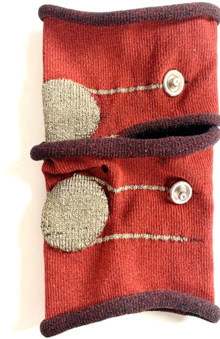
Figure 16 - Image depicting the tube iteration of Prototype 2. With copper stitched EMG electrodes and button connectors visible.
