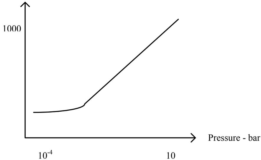
Figure 3.10: Graph showing breakdown voltage versus pressure for SF<sub>6</sub>
