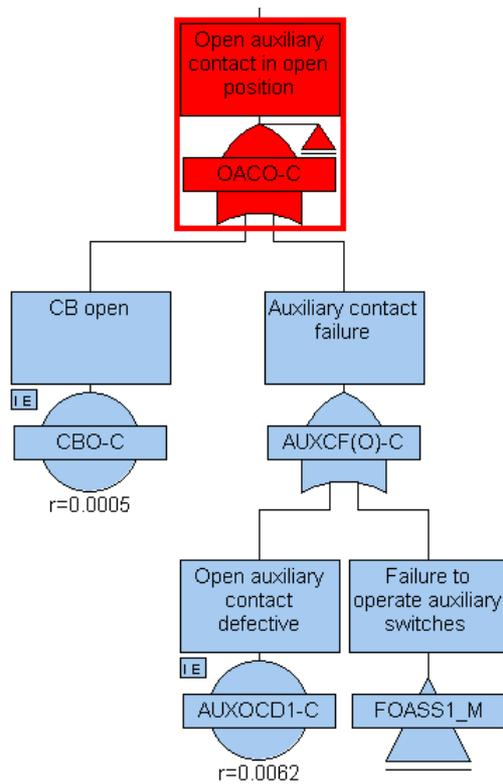
Figure 6.37: FTD for auxiliary switch contact failure
