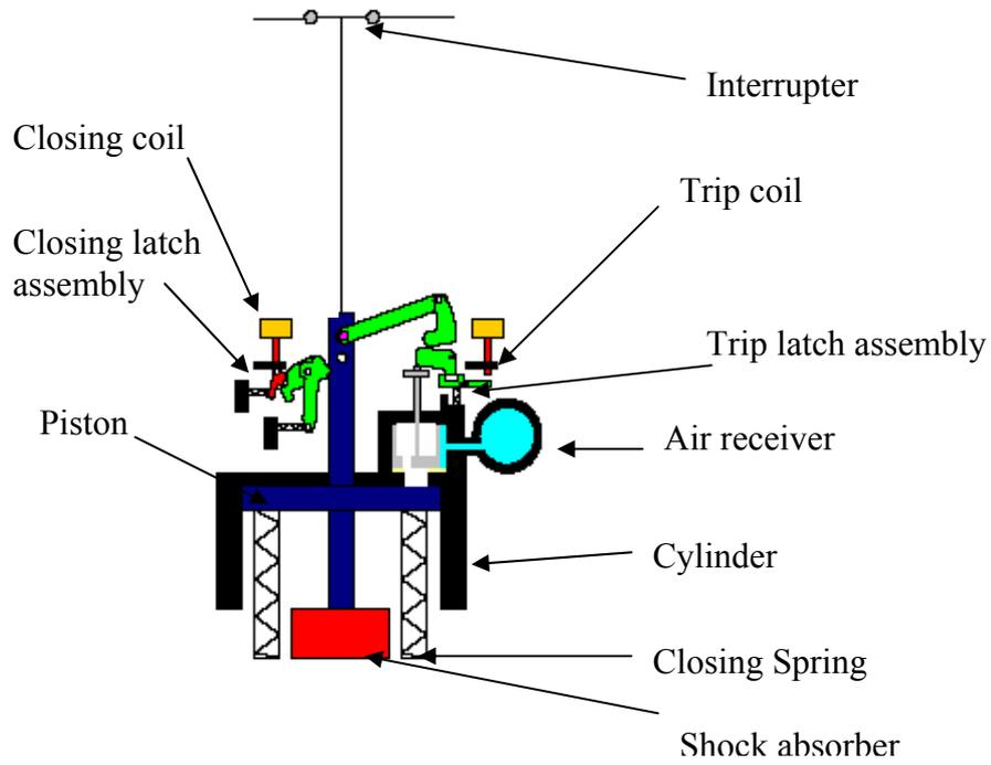
a) Mechanism in closed position
