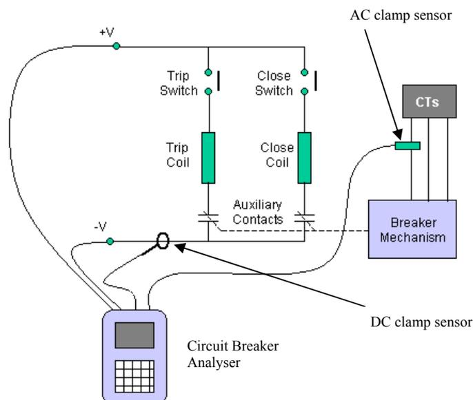
Figure 2.20: Diagram showing the non-invasive connection of a circuit breaker analyser to evaluate the condition of an operating mechanism<sup>6</sup>
