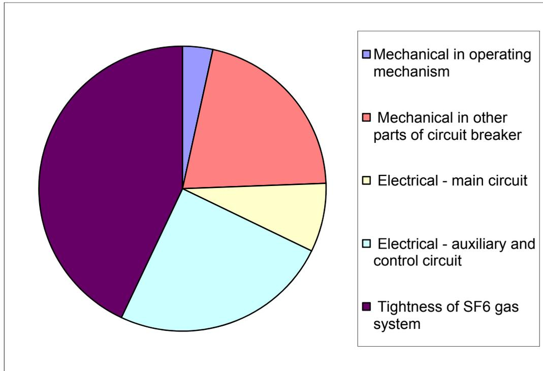
Figure 6.41: Diagram showing the origin of metal enclosed circuit breaker failures, utilizing a spring mechanism, from an international survey<sup>20</sup>
