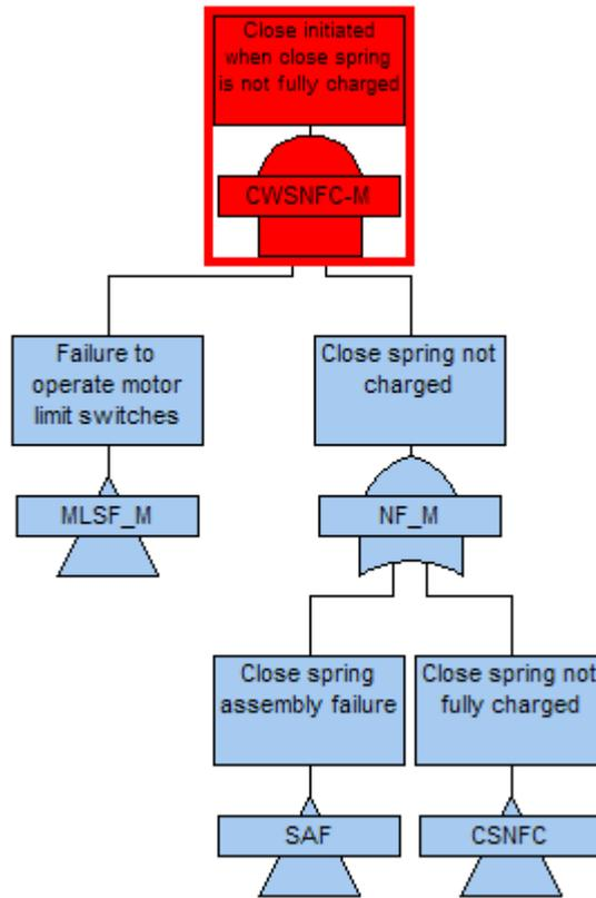
Figure 6.10: FTD for close operation initiated when spring is not fully charged
