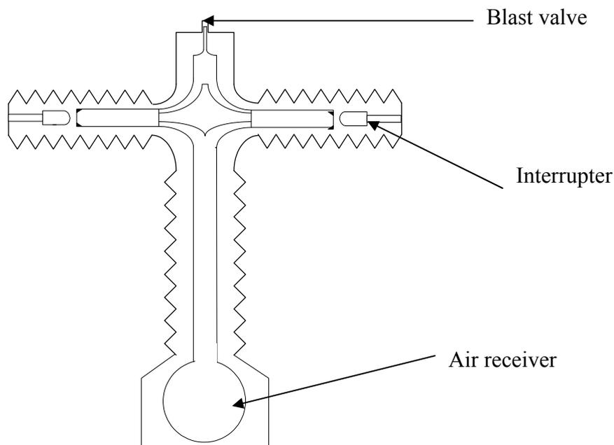
Figure 2.9: Schematic showing an ABCB fully pressurized head design
