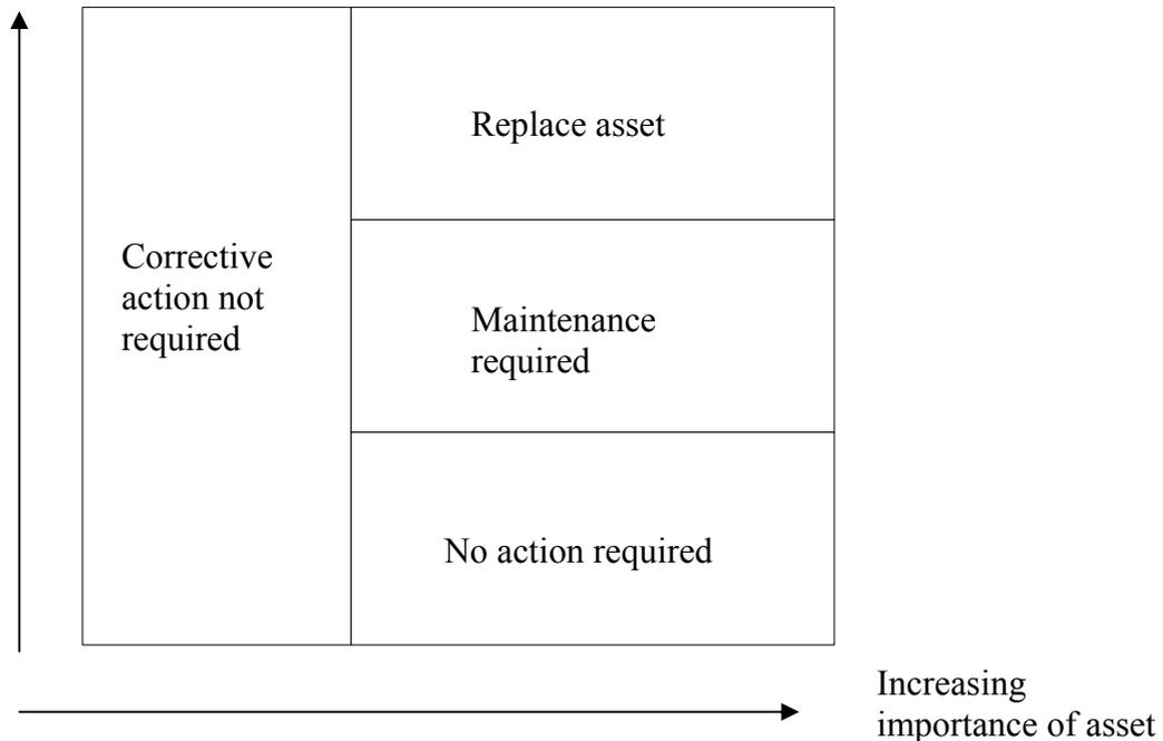
Figure 2.24: Diagram showing a decision making map for maintenance action<sup>10</sup>
