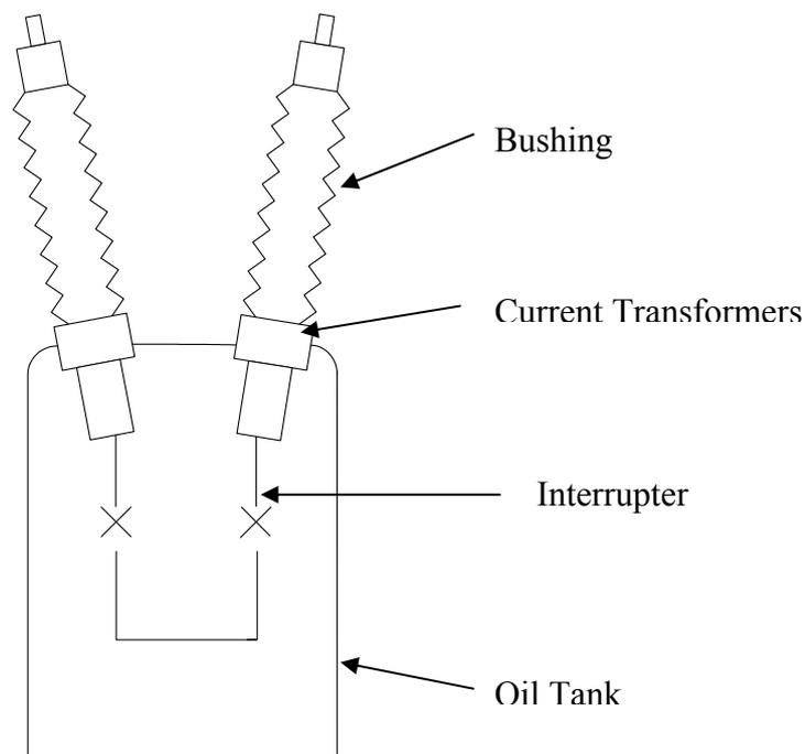
Figure 2.5: Schematic showing a single phase of a High Voltage (HV) bulk oil circuit breaker
