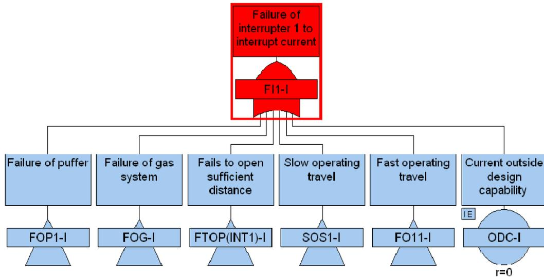
Figure 6.18: FTD for failure of interrupter chamber
