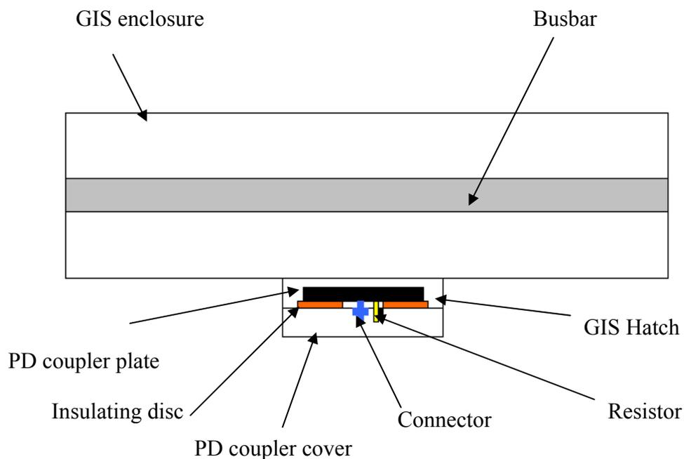
Figure 4.4: Diagram showing a typical PD coupler design
