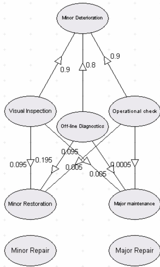
Figure 7.10: Off-line CBM Markov model showing outcome from off-line diagnostic checks
