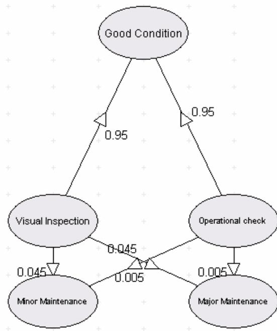
Figure 7.5: TBM Markov model showing outcome from visual inspection and operational check
