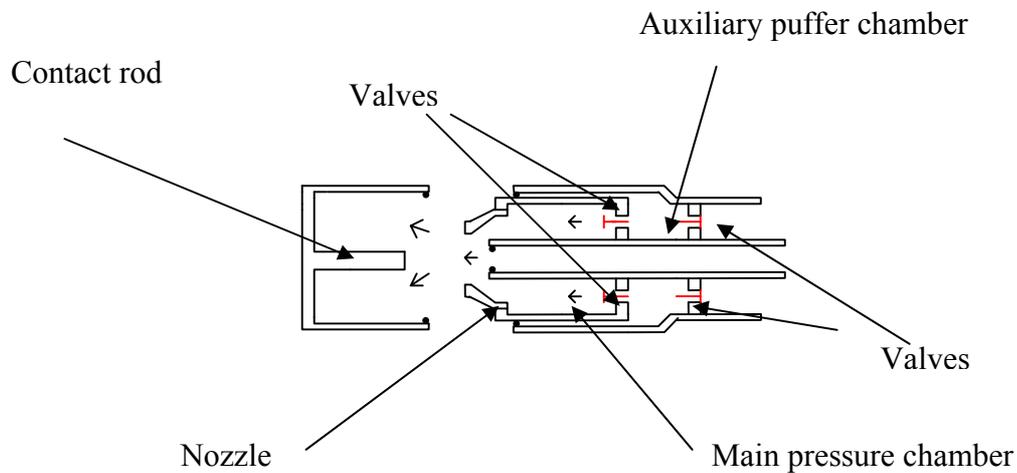
Figure 2.16: Diagram showing the self blast or auto puffer interrupter principle of operation
