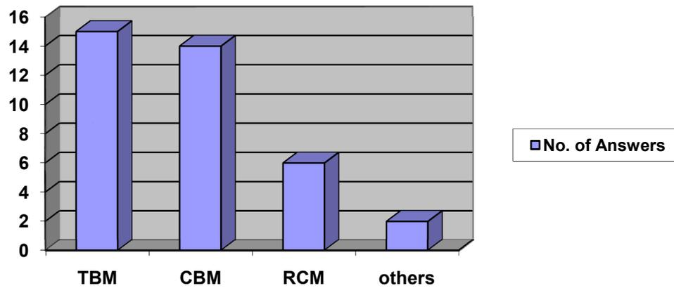
Figure 2.4: Results of a survey showing maintenance methods currently employed for circuit breakers<sup>4</sup>
