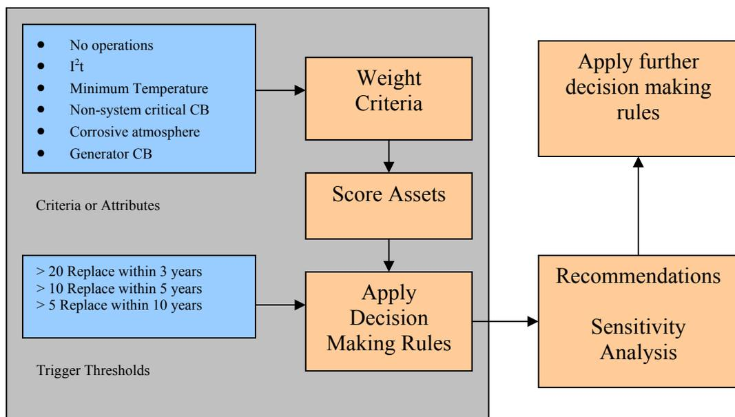
Figure 8.1: Diagram showing multiple criteria decision making for prioritizing the replacement/refurbishment of circuit breakers
