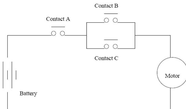
Figure 6.2: Electrical schematic for a motor circuit
