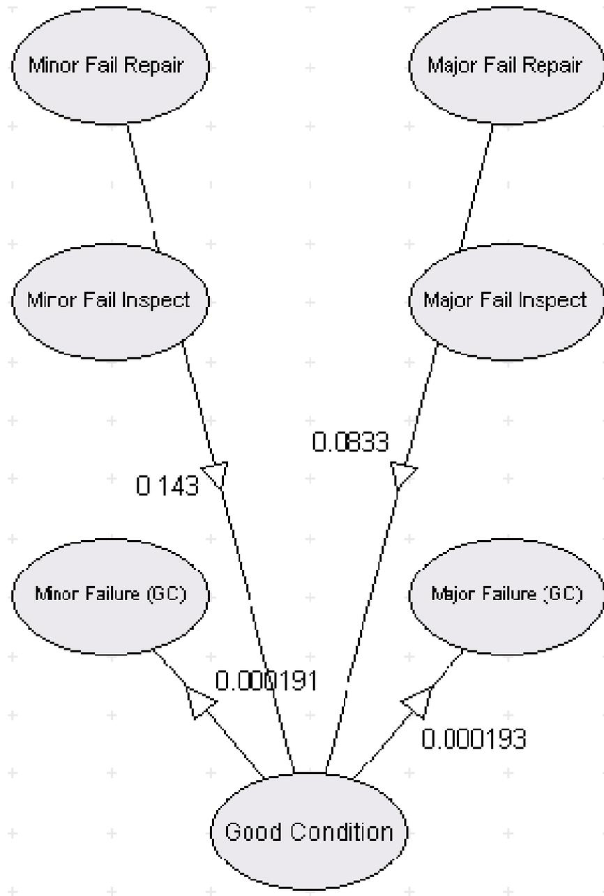
Figure 7.7: TBM Markov model showing minor and major failures
