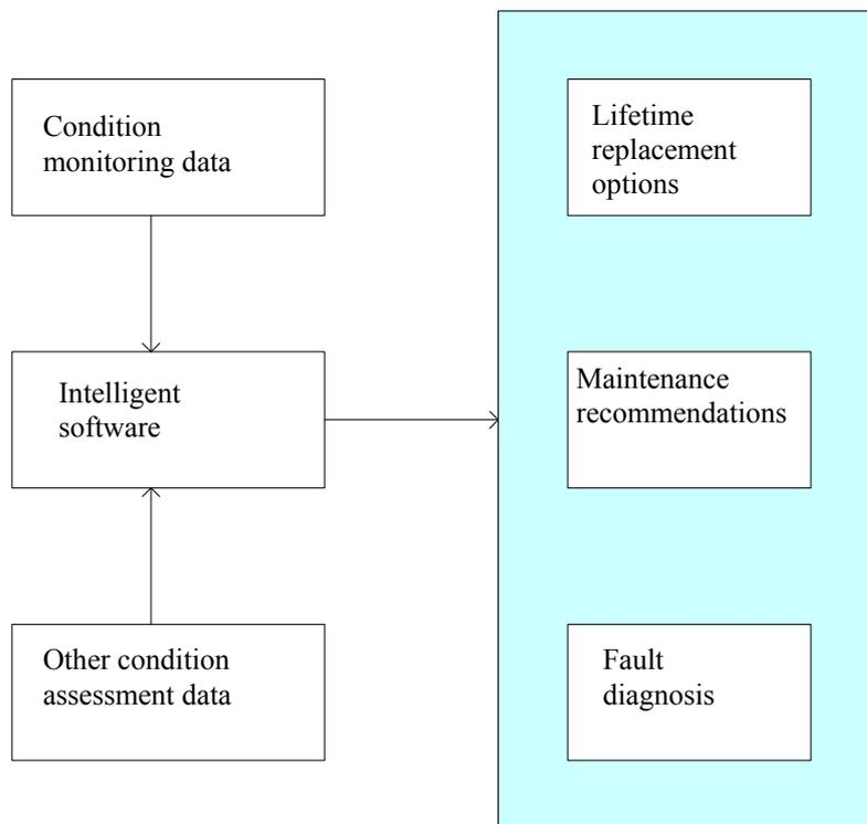
Figure 3.3: Diagram showing a plant asset management model
