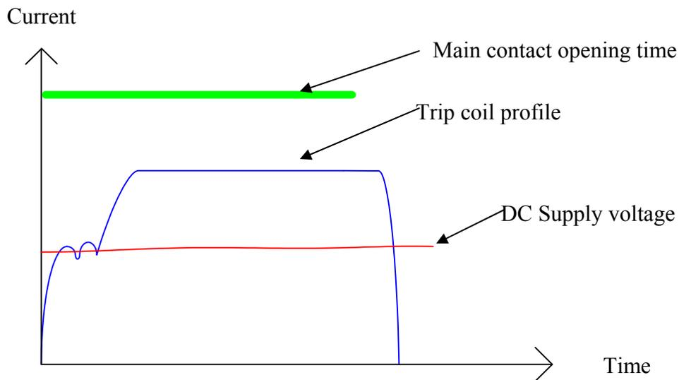
Figure 2.21: Diagram showing a typical circuit breaker operating signature<sup>7</sup>
