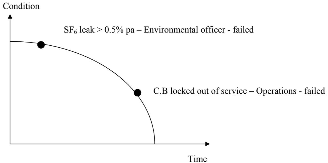
Figure 5.2: Diagram showing the different stages of failure recognition depending on user's perspective
