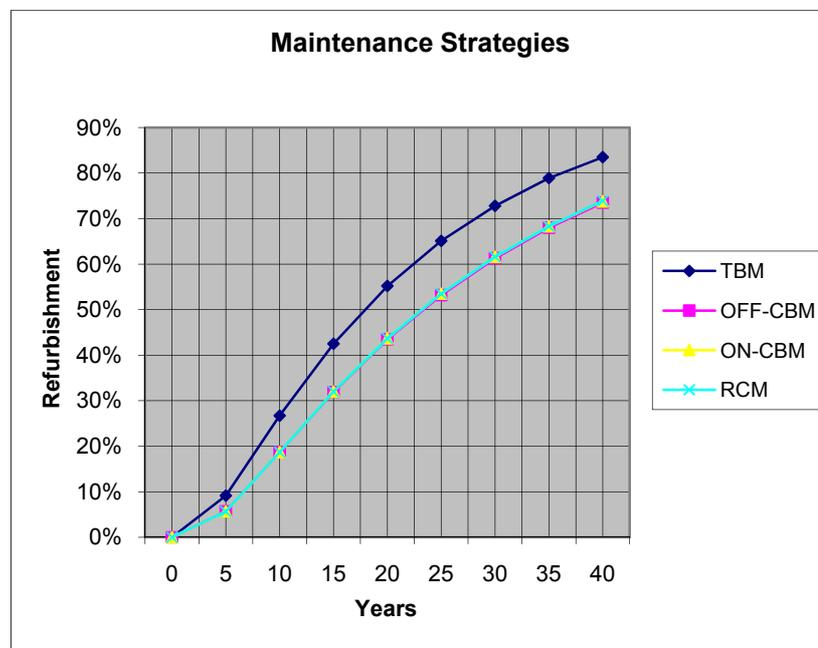
Figure 7.15: Graph showing probability of a circuit breaker requiring refurbishment versus years in service for each maintenance strategy
