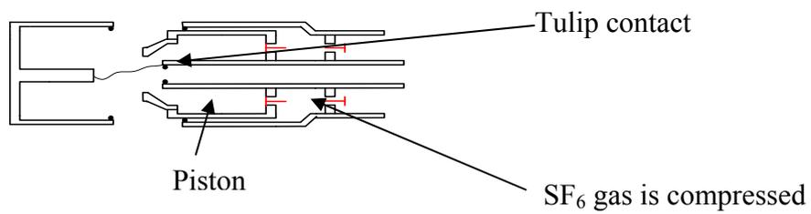
b - Arc burn between contact rod and tulip contact
