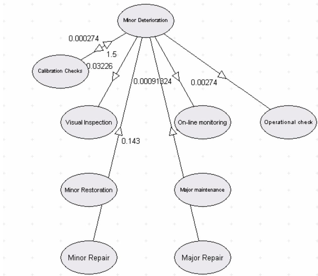
Figure 7.11: On-line CBM Markov model showing monitoring and maintenance activities
