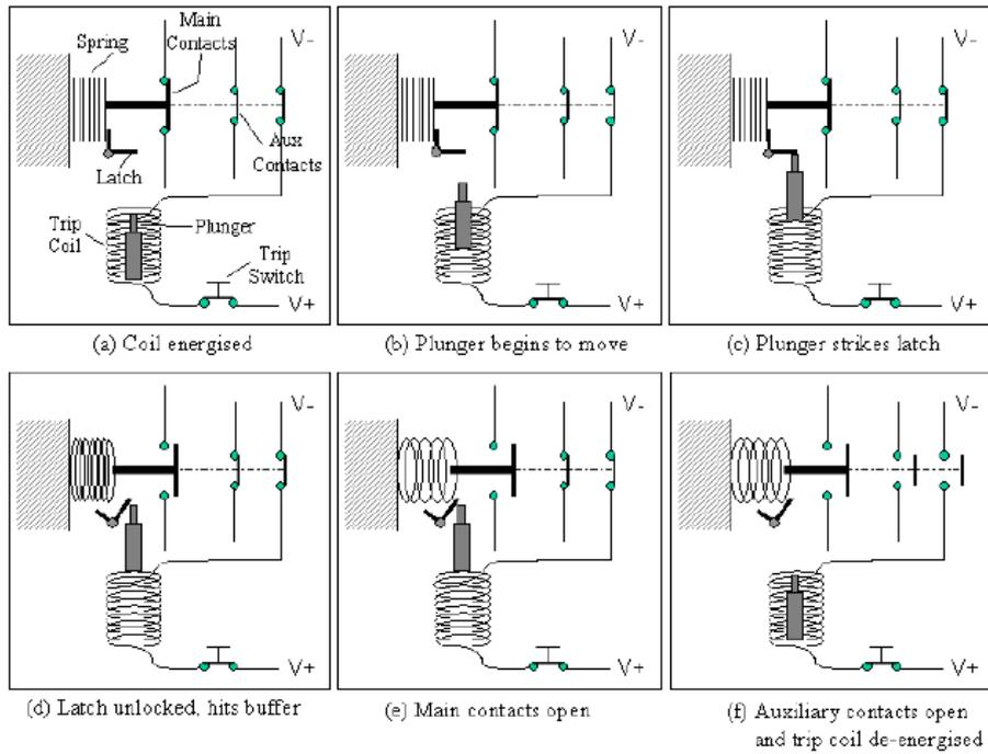
Figure 3.4: Diagram showing the energisation and movement stages of the trip solenoid during the opening sequence of a circuit breaker<sup>12</sup>
