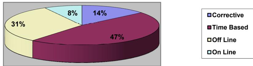
Figure 2.3: Results of a survey showing the maintenance strategies used by transmission and distribution utilities<sup>3</sup>
