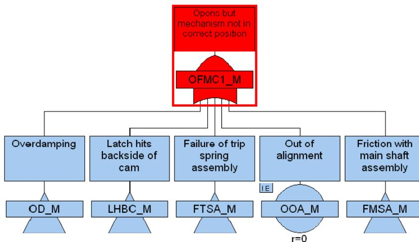
Figure 6.5: Top level FTD for failure mode 'opens but mechanism not in the correct position'
