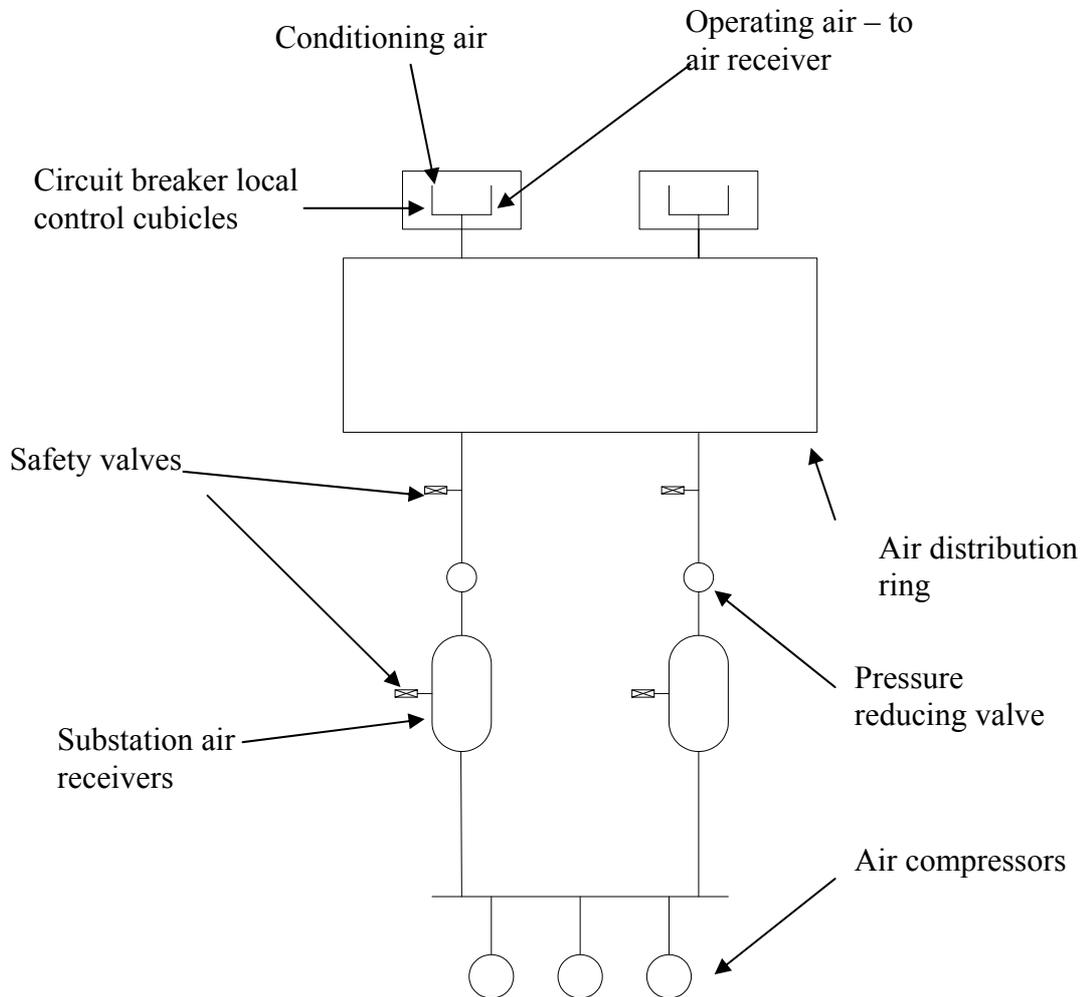
Figure 2.7: Schematic showing a typical ABCB compressed air system
