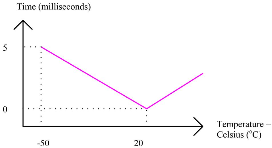
Figure 3.9: Diagram showing how a circuit breaker operating time can vary with temperature<sup>14</sup>
