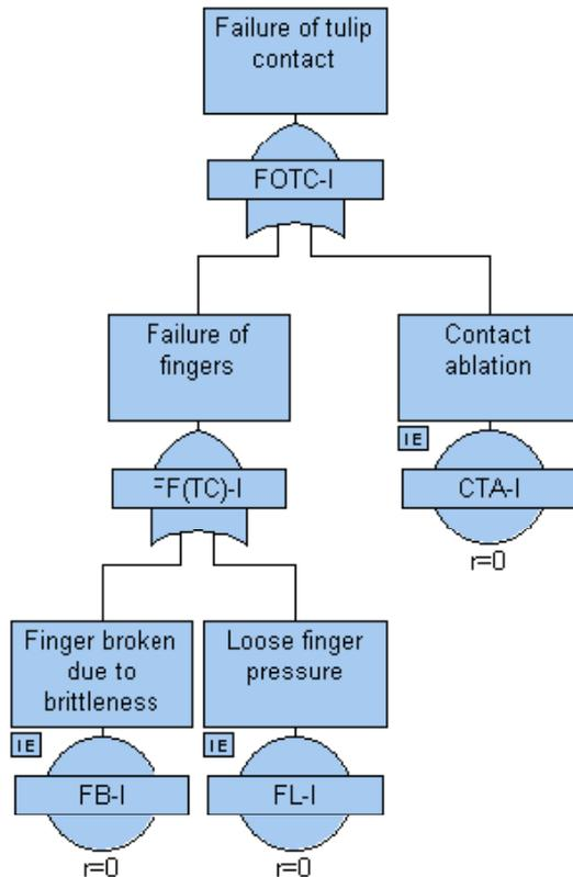
Figure 6.22: FTD for failure of tulip contact
