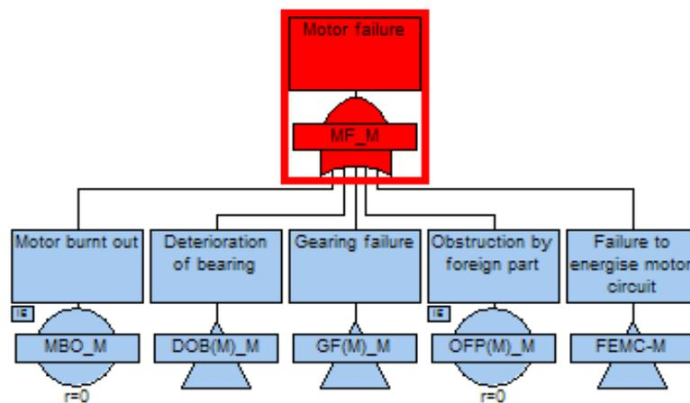
Figure 6.14: FTD for the motor failure
