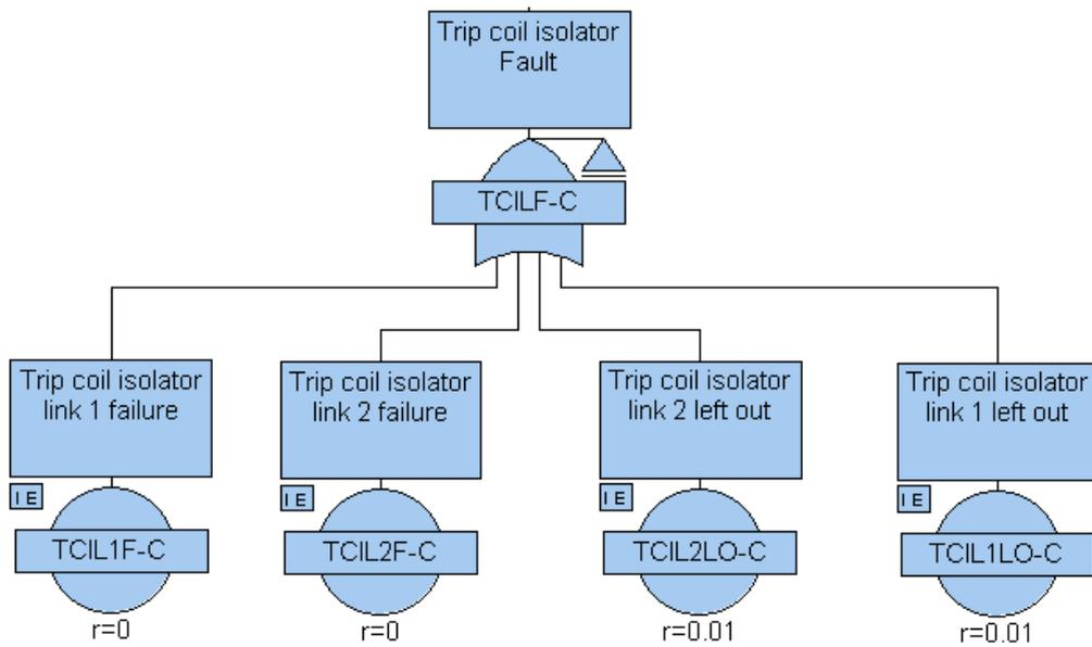
Figure 6.36: FTD for trip coil isolation fault
