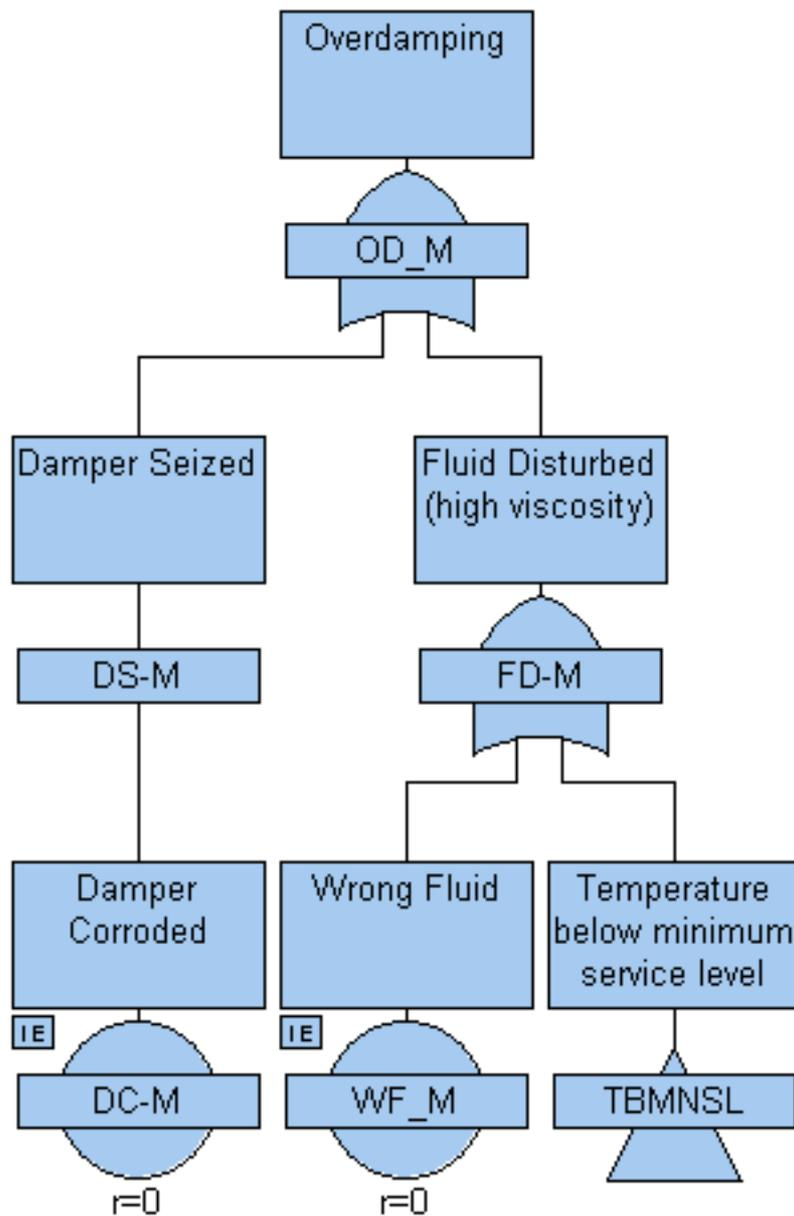
Figure 6.6: FTD for overdamping
