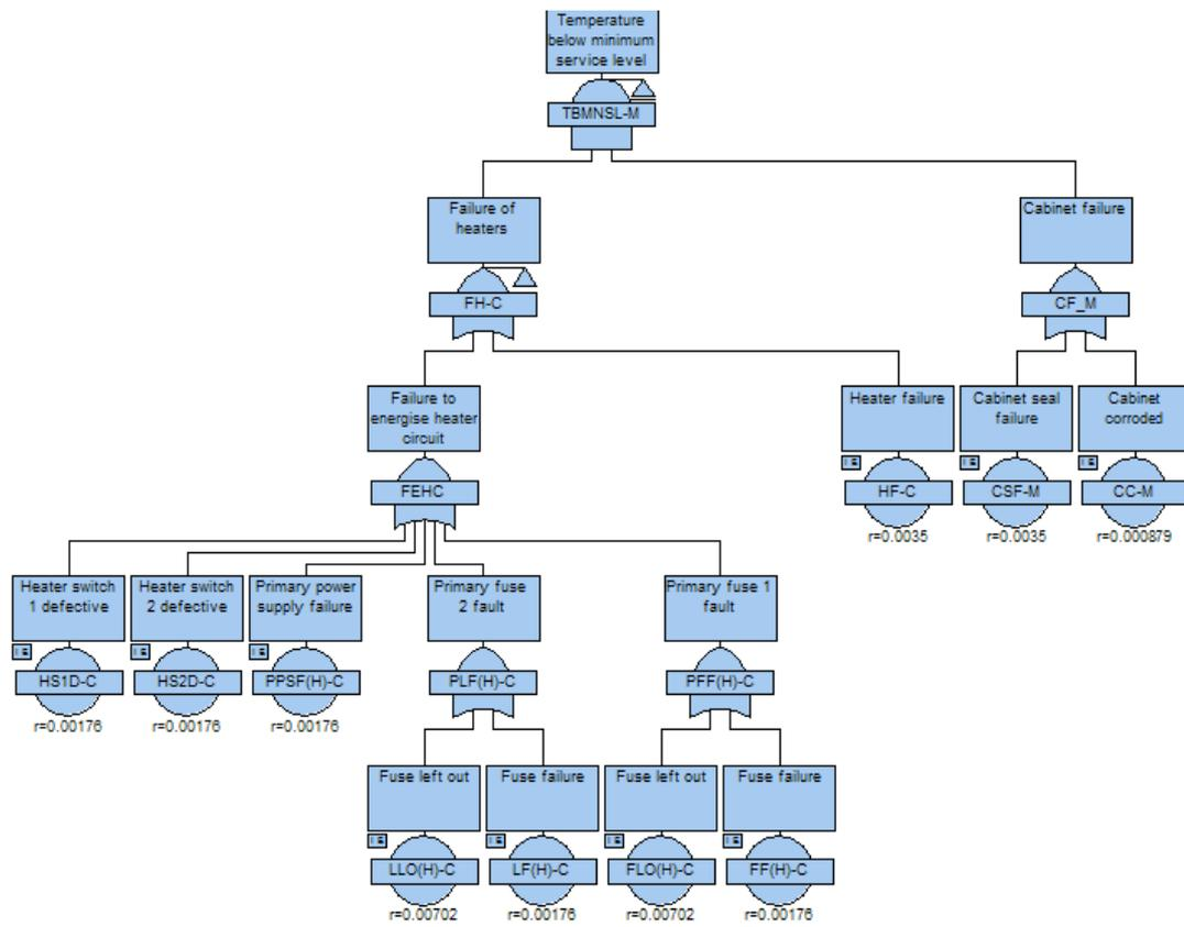
Figure 6.7: FTD for temperature below minimum service level
