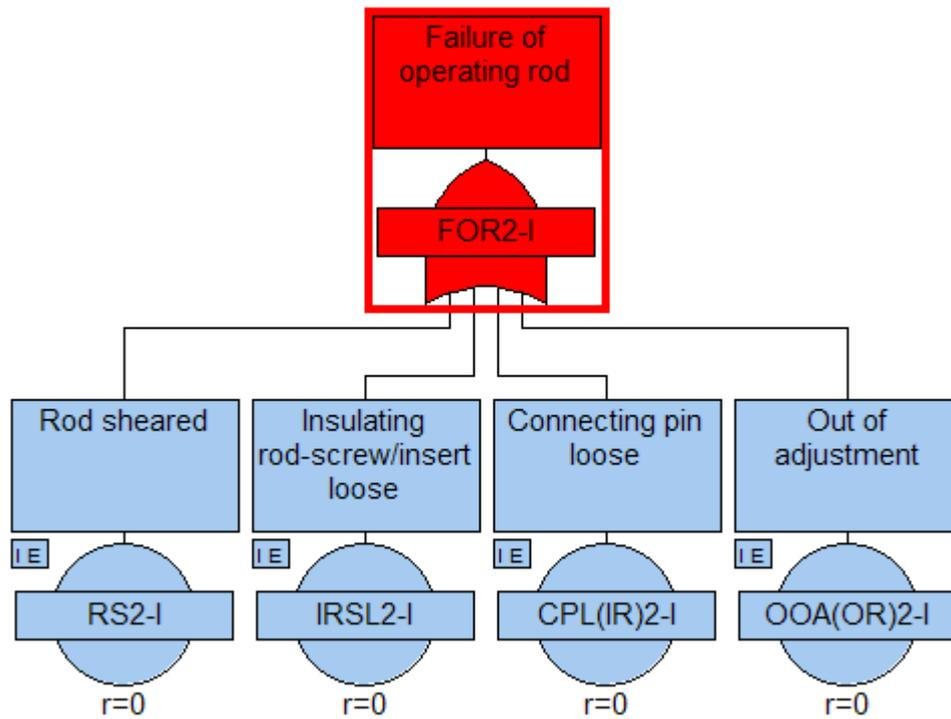
Figure 6.23: FTD for failure of operating rod
