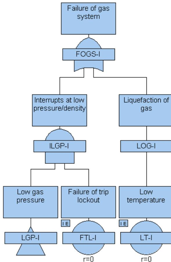
Figure 6.24: FTD for failure of the gas system
