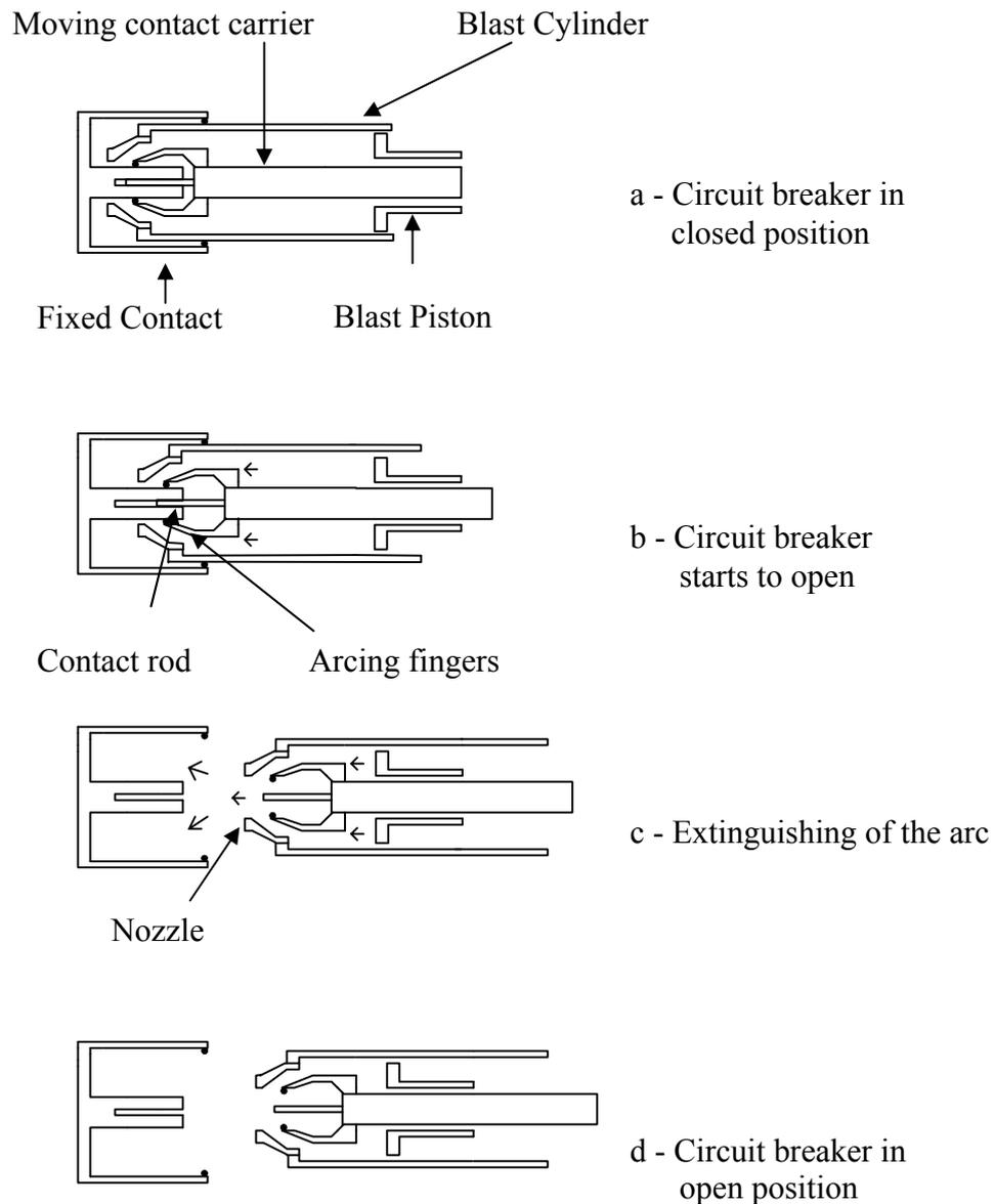
Figure 2.14: Diagram showing the single pressure 'puffer' interruption technique
