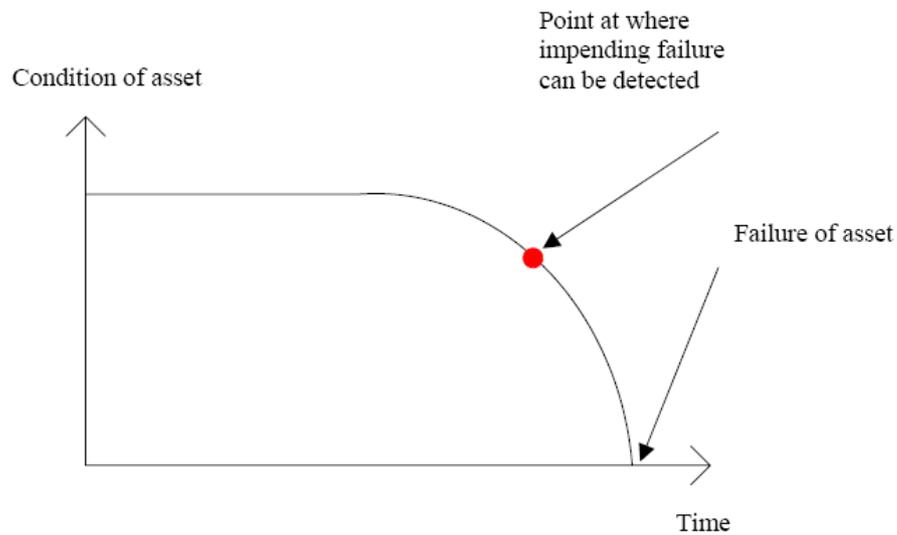
Figure 3.1: Diagram showing how a failure starts and progresses to the point where it can be detected
