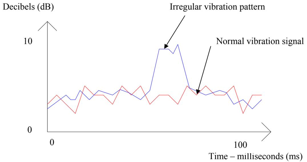
Figure 3.13a: Graph showing the deviation in amplitude versus time from the vibration analysis of a circuit breaker opening signal<sup>16</sup>
