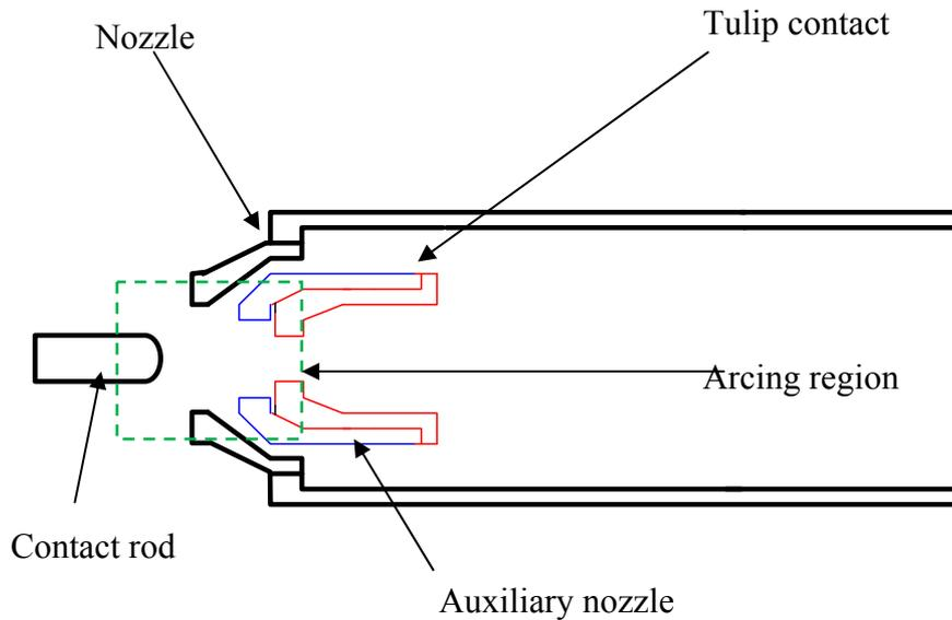
Figure 6.21: Diagram showing electrical arcing within the interruption chamber
