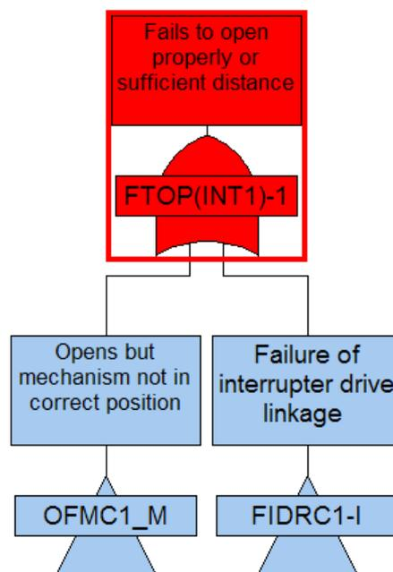
Figure 6.29: FTD for interrupter fails to open sufficiently
