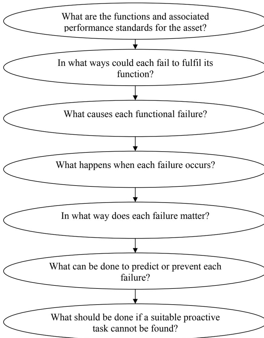
Figure 5.1: Diagram showing the seven steps to RCM
