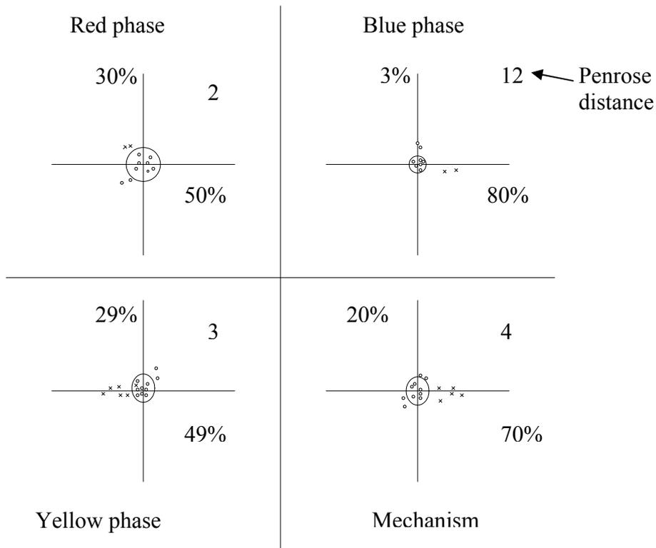
Note: Normal operation for red and yellow phases, with a fault existing on the blue phase.
