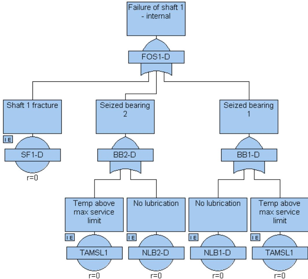
Figure 6.32: FTD for failure of drive shaft operating shaft
