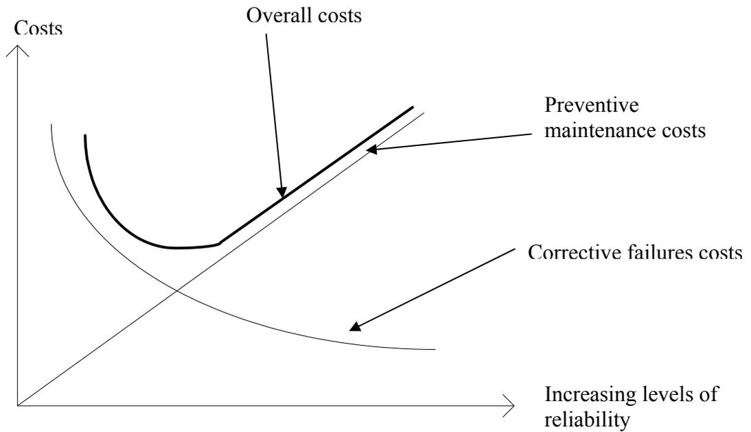
Figure 2.1: Maintenance and failure costs versus investment cost to improve reliability
