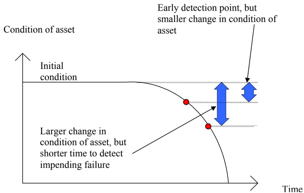
Figure 3.2: Diagram showing how change in condition of an asset varies with time <sup>11</sup>
