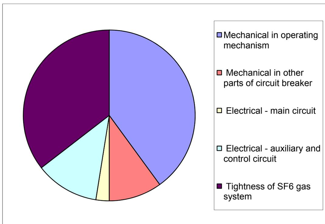
Figure 6.40: Diagram showing the origin of circuit breaker failures from an international survey<sup>19</sup>
