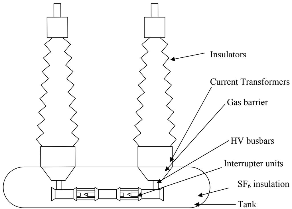
Figure 2.10: Schematic showing a single phase of an SF<sub>6</sub> dead tank circuit breaker
