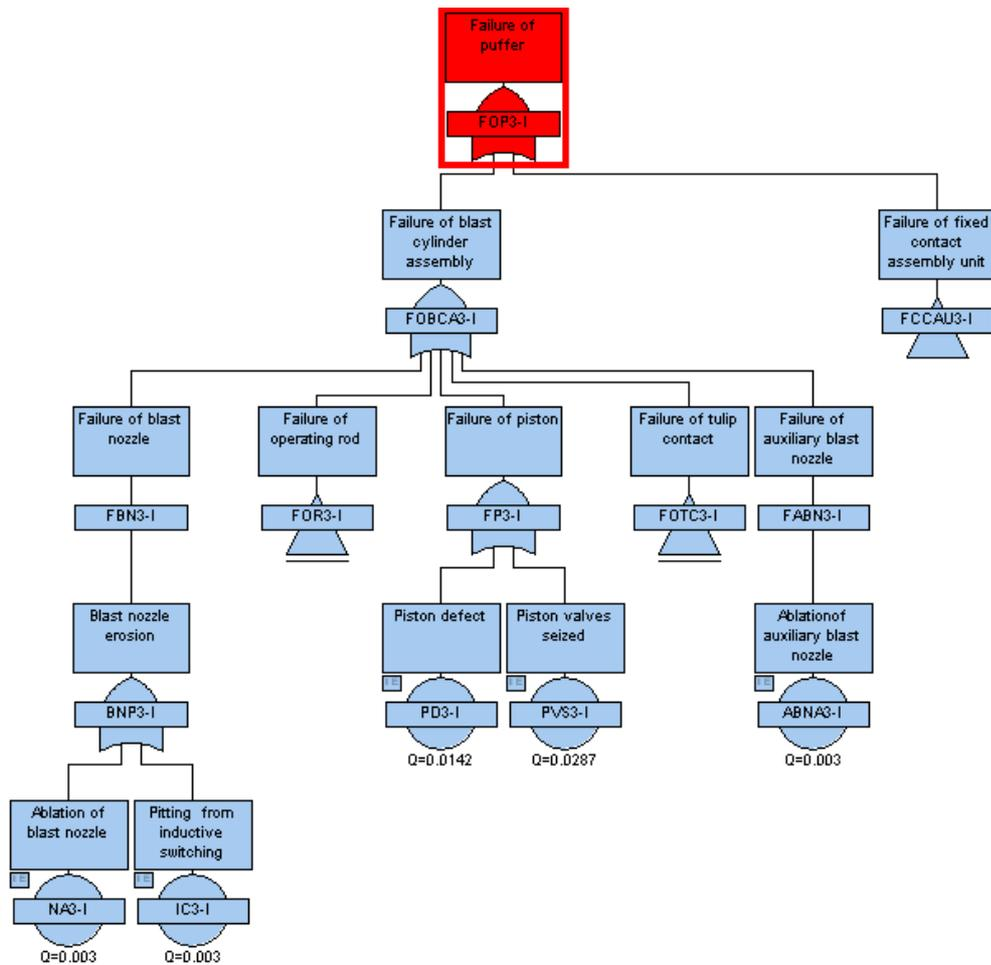
Figure 6.19: FTD for failure of the blast cylinder assembly and fixed contact assembly unit.
