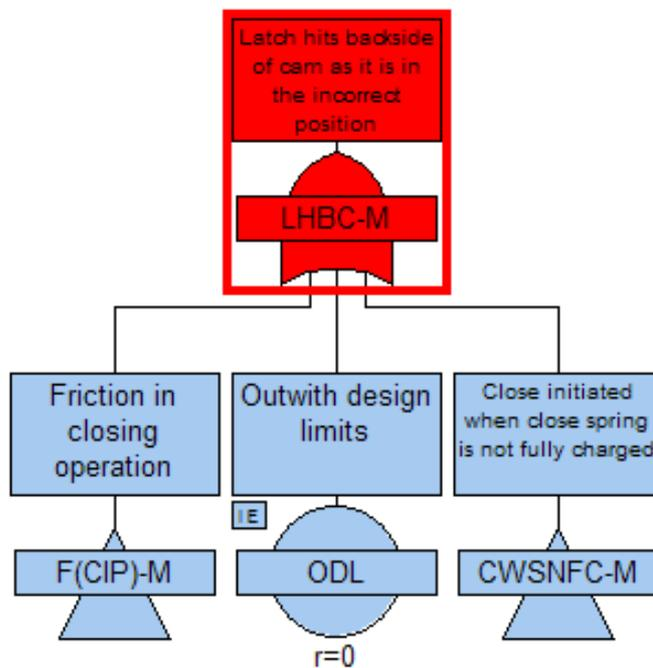
Figure 6.8: FTD for latch hits backside of cam
