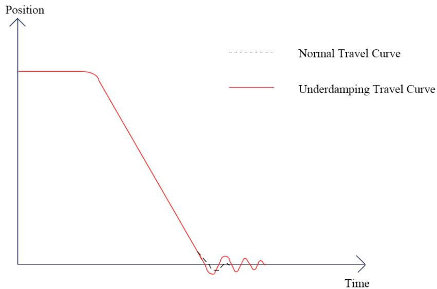
Figure 3.7: Diagram of a circuit breaker travel curve showing underdamping
