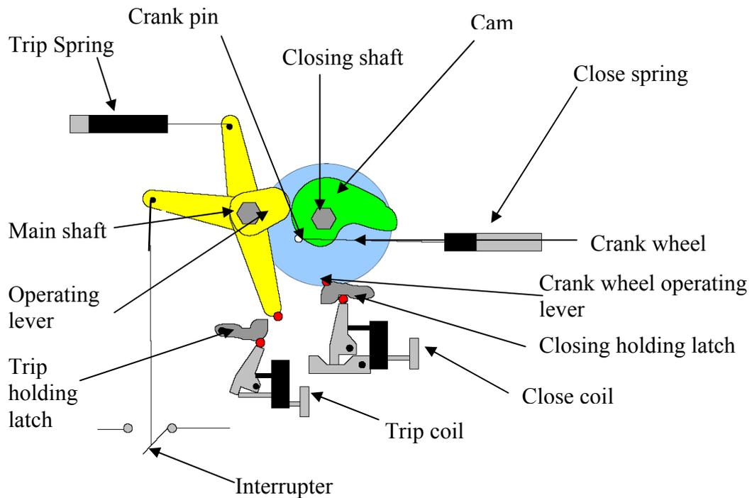
Figure 6.4: Diagram of a spring type operating mechanism
