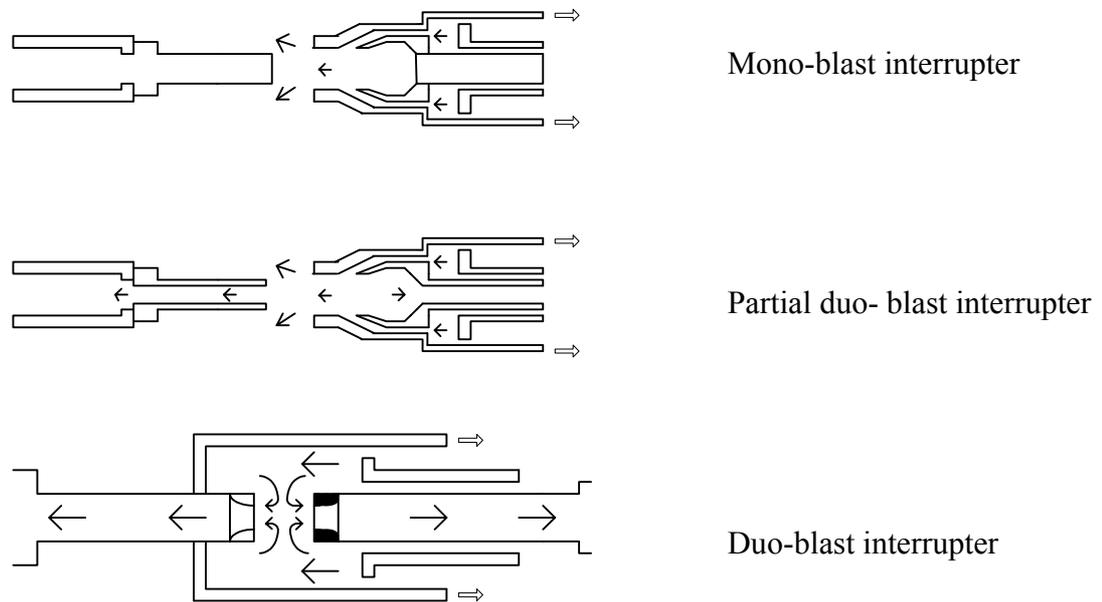
Figure 2.15: Diagram showing different categories of SF<sub>6</sub> puffer interrupters
