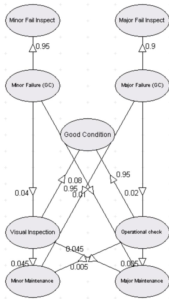
Figure 7.8: TBM Markov model showing outcome from minor and major failures
