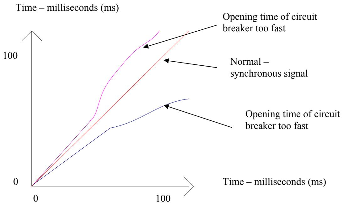
Figure 3.13b: Graph showing the deviation in time from the vibration analysis of a circuit breaker opening signal<sup>17</sup>
