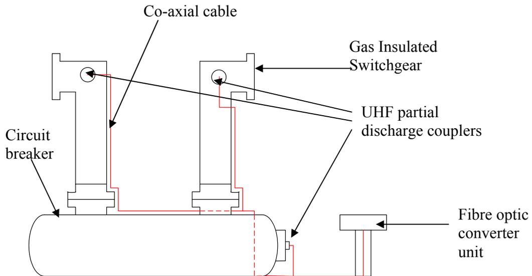
Figure 3.11: Diagram of a typical partial discharge monitoring system for GIS
