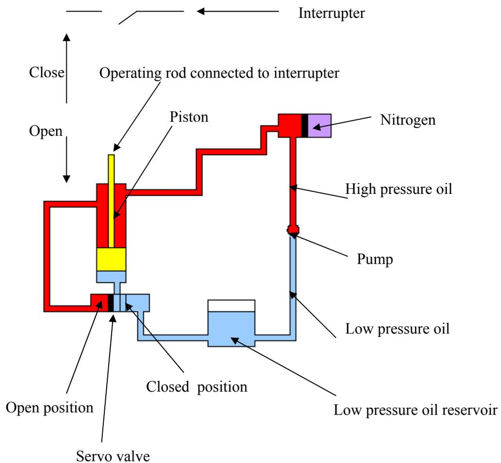
Figure 2.18: Diagram showing the operating principle of a hydraulic type mechanism
