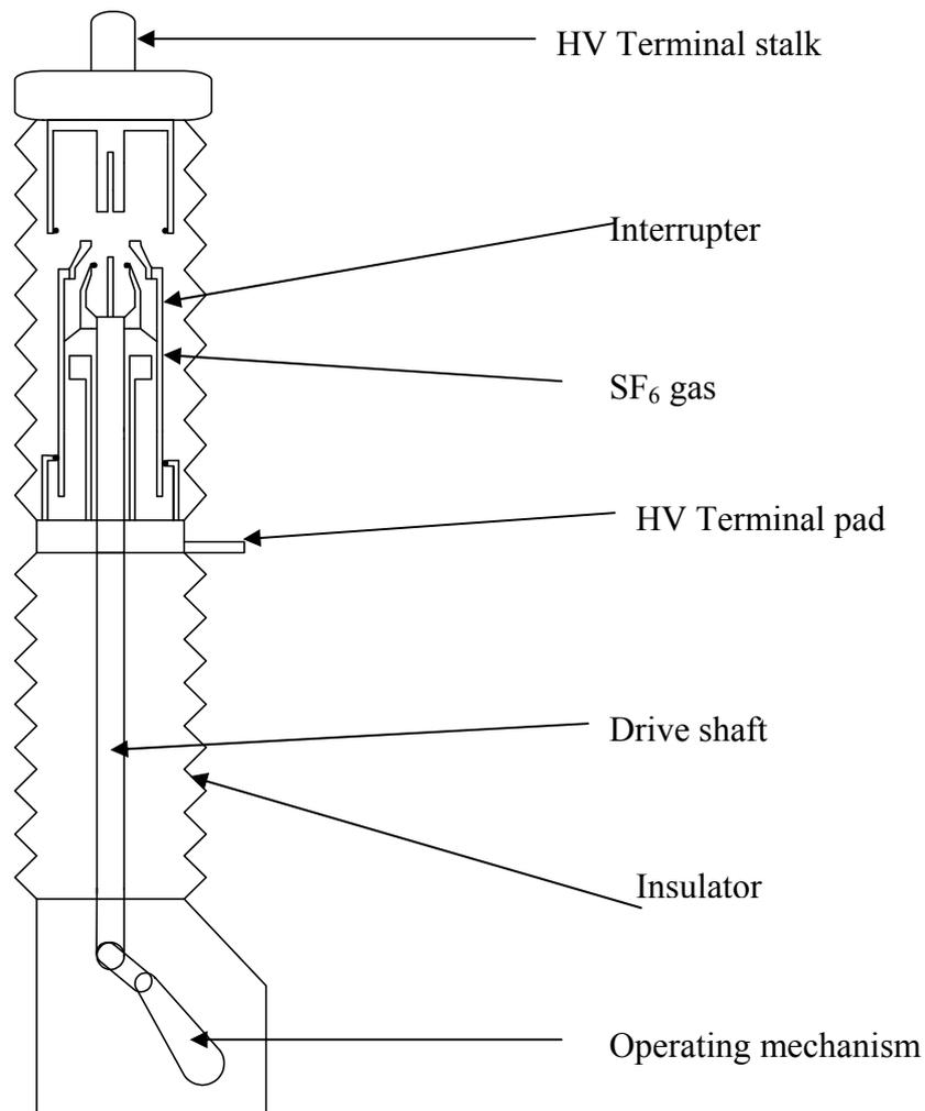
Figure 2.12: Schematic showing a single phase of an SF<sub>6</sub> air insulated or live tank circuit breaker
