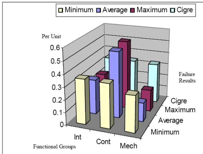
Figure 6.43: Comparison of FTA circuit breaker functional group failure contributions with the results from an international survey for metal enclosed circuit breaker spring mechanism failures when filtered to reduce the number of SF<sub>6</sub> leakage failures<sup>22</sup>
