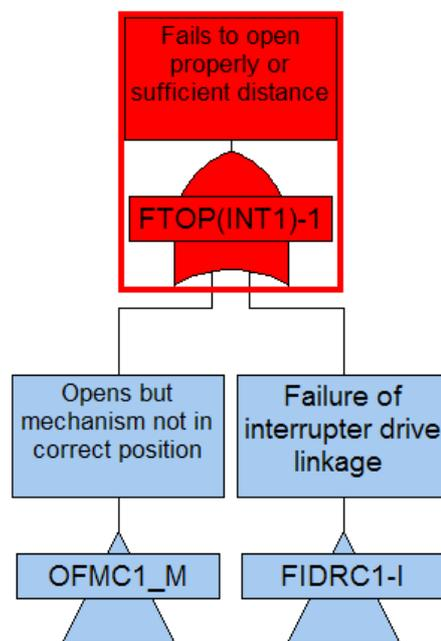
Figure 6.29: FTD for interrupter fails to open sufficiently
