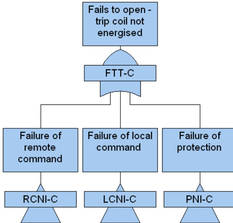
Figure 6.33: FTD for fails to open – trip coil not energized
