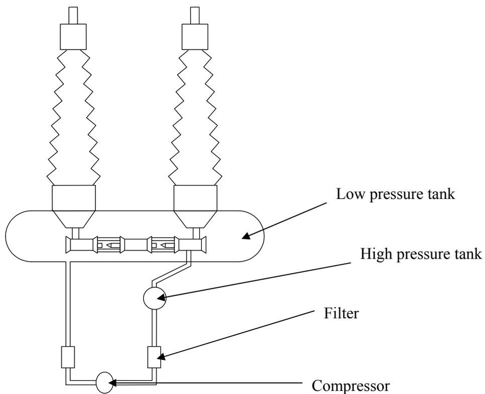
Figure 2.13: Schematic showing a double pressure SF<sub>6</sub> circuit breaker
