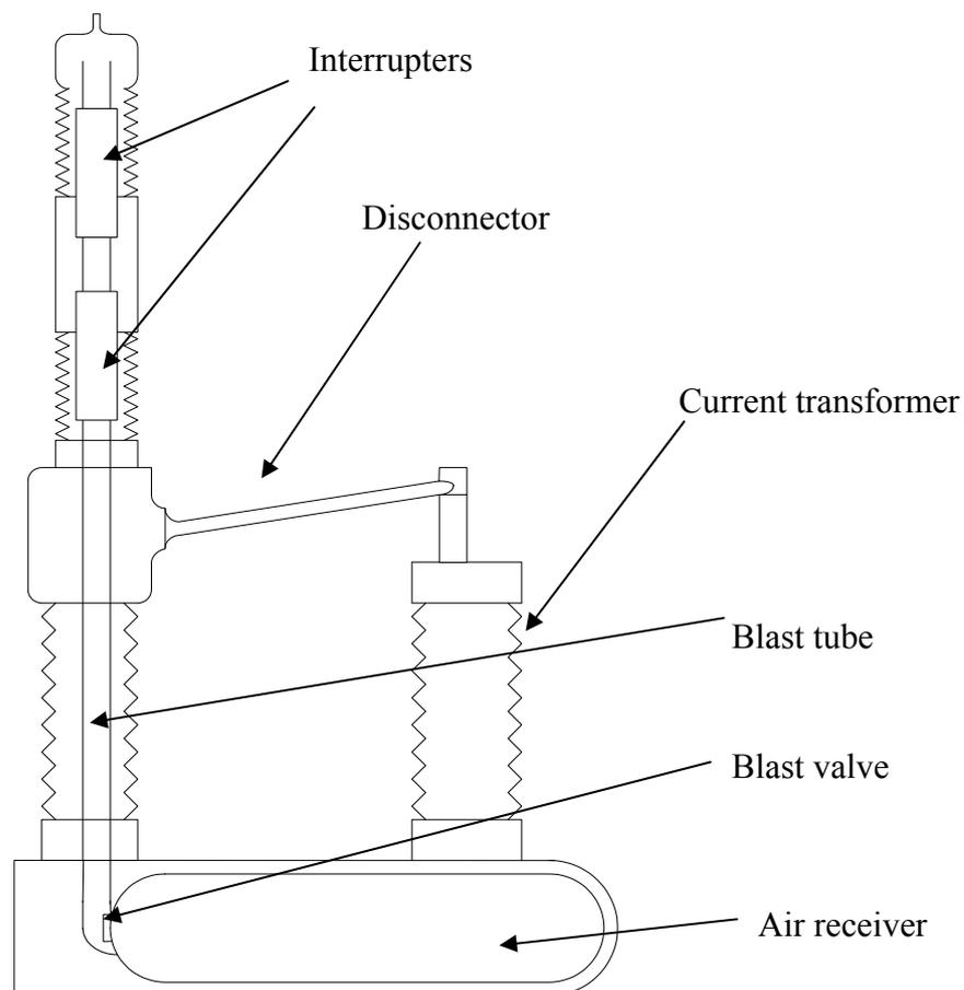
Figure 2.8: Schematic showing an ABCB non-pressurized head design
