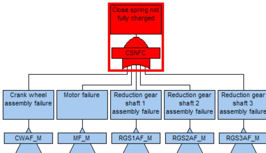
Figure 6.12: FTD for close spring not fully charged
