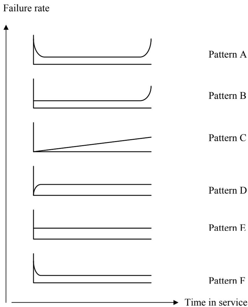
Figure 2.2: Diagram showing different types of equipment failure patterns<sup>2</sup>
