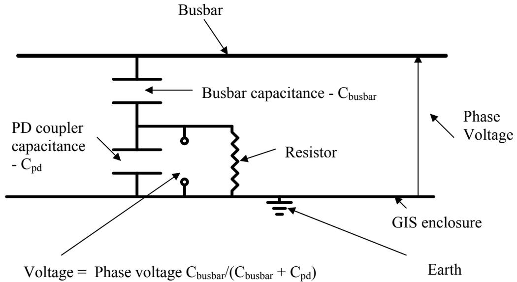
Figure 4.5: Diagram showing the PD coupler principle of operation
