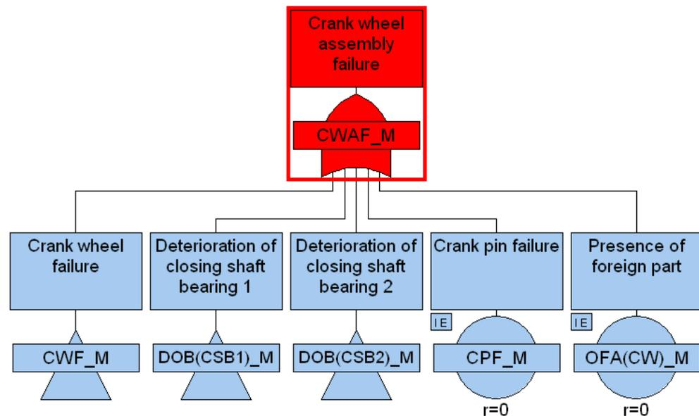
Figure 6.16: FTD for failure of the crank wheel assembly
