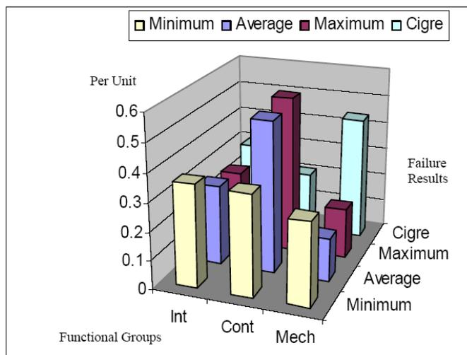
Figure 6.42: Comparison of FTA results with the results from an international survey for metal enclosed circuit breaker failures, utilizing a spring mechanism<sup>21</sup>
