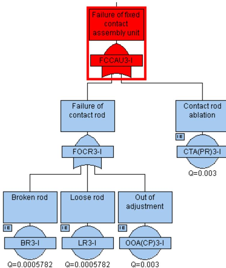
Figure 6.20: FTD for the fixed contact assembly unit
