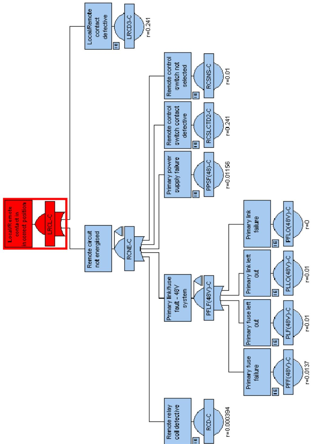
Figure 6.35: FTD for local/remote contact in incorrect position
