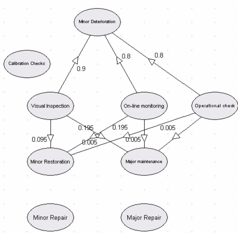
Figure 7.12: On-line CBM Markov model showing outcome from on-line condition monitoring checks
