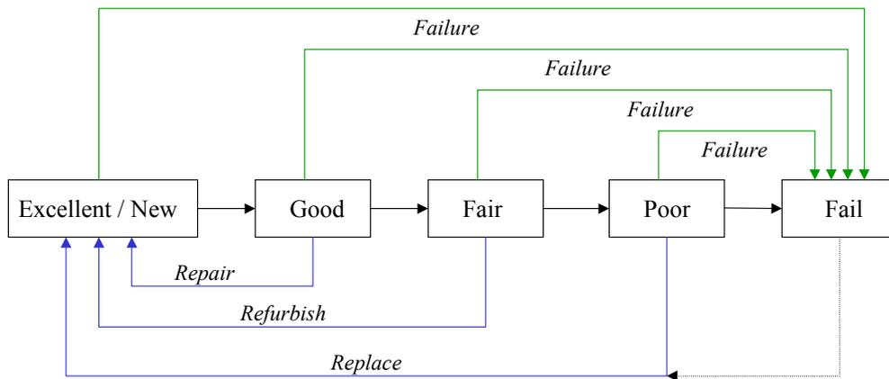
Figure 8.2: Diagram showing multiple criteria decision making to optimize the investment plan for a circuit breaker
