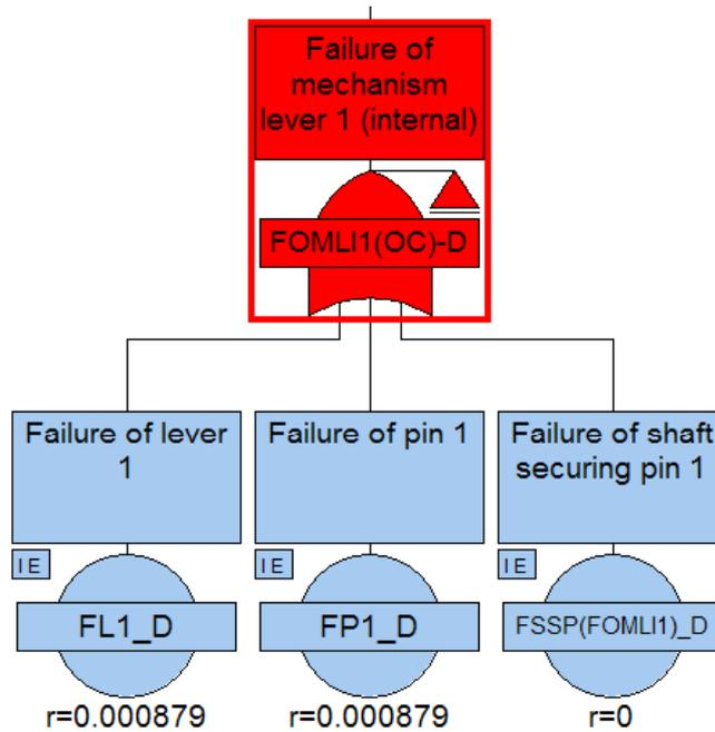
Figure 6.31: FTD for failure of drive linkage lever
