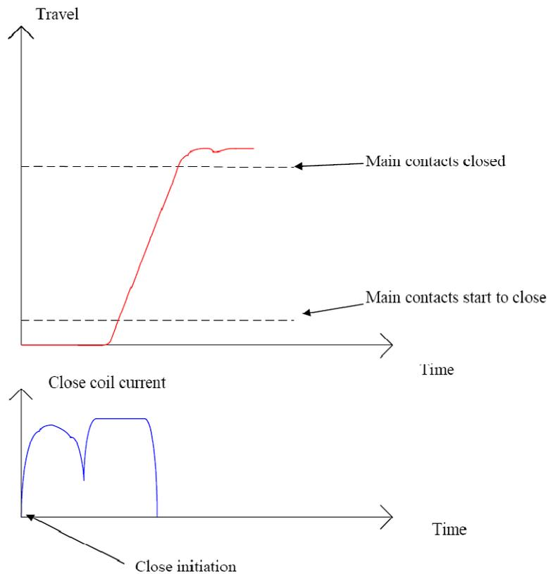
Figure 3.8: Diagram of a typical circuit breaker closing travel curve
