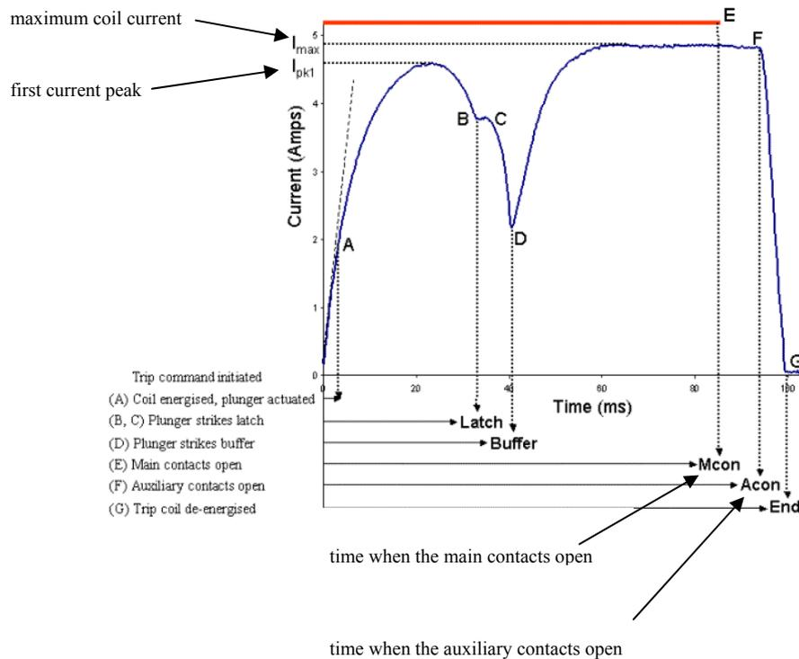
Figure 3.5: Diagram showing a typical circuit breaker trip coil current signature<sup>13</sup>
