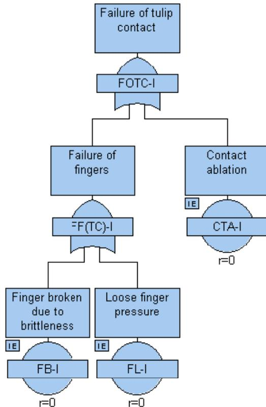
Figure 6.22: FTD for failure of tulip contact
