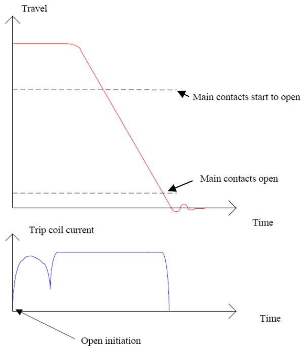
Figure 3.6: Diagram showing a typical circuit breaker opening travel curve
