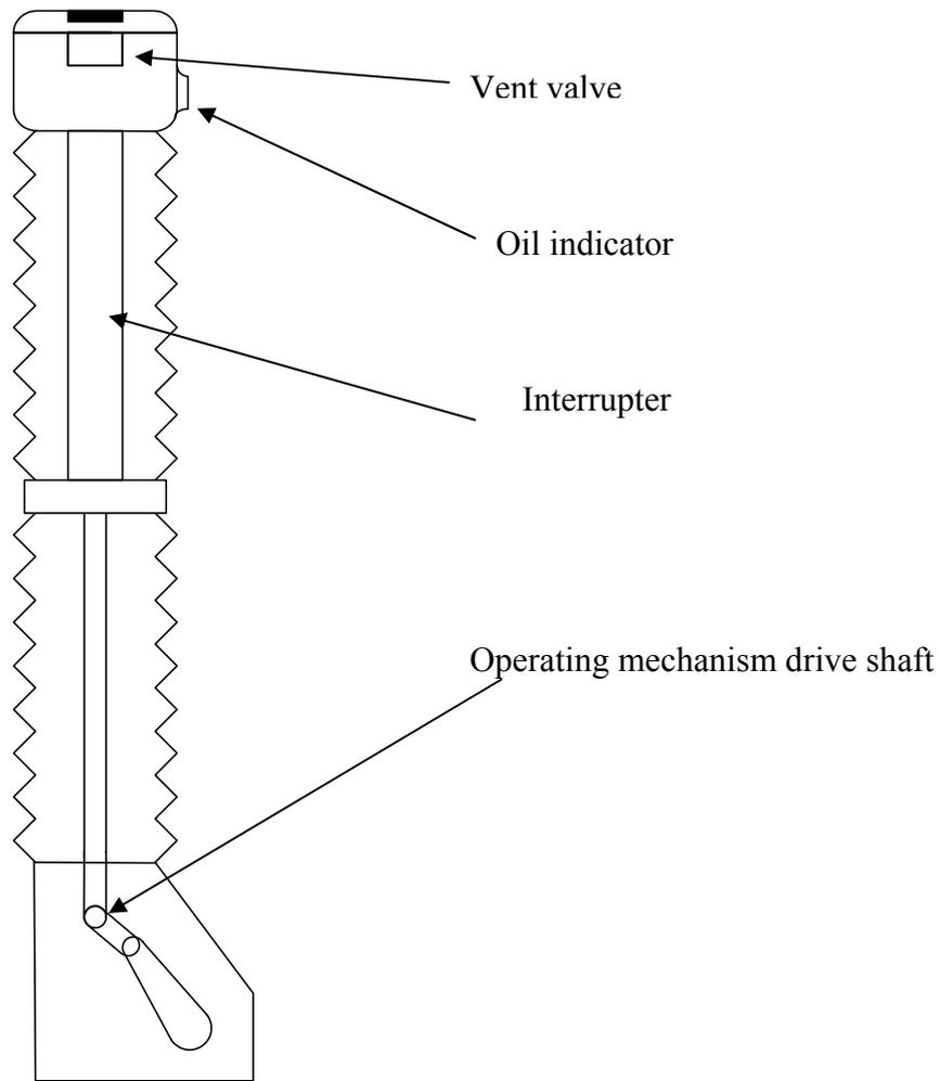
Figure 2.6: Sectional view of one pole of a minimum or small oil circuit breaker
