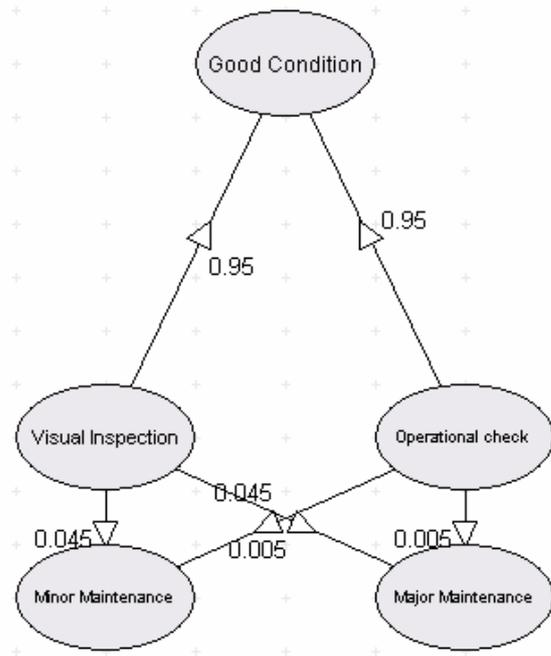
Figure 7.5: TBM Markov model showing outcome from visual inspection and operational check
