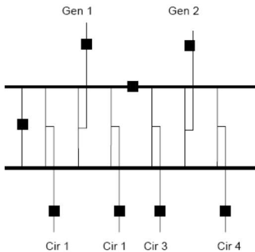
Figure 4.3: Diagram showing a double busbar substation configuration
