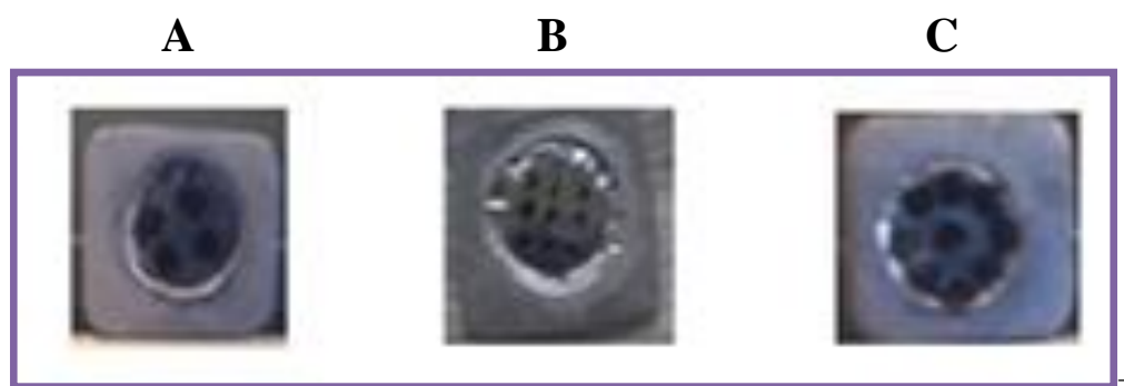
Figure 6.3 Examples of patterned AuNR samples produced using PTFE masks. Sample A – four 1.25 mm dots, sample B – nine 0.5 mm dots and sample C – nine 1 mm dots.
