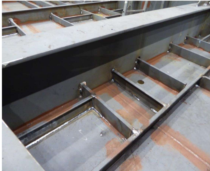
Figure 1-10 Example of a welded panel assembly used in ship construction
