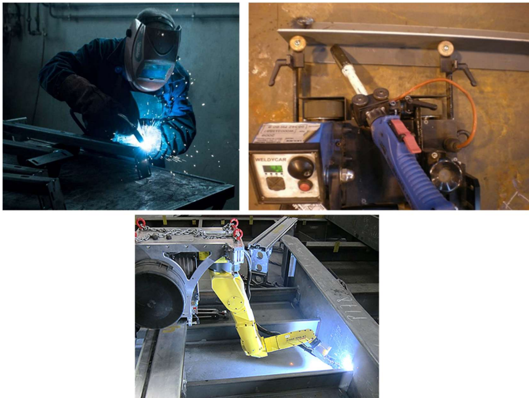
Figure 1-3 Examples of Manual, Semi-Automatic 'Weldy Car' and Robotic welding
