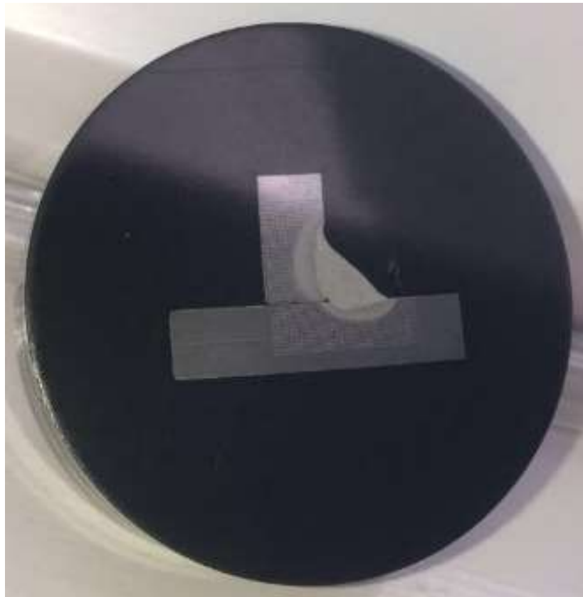
Figure 3-25 Example polished test piece used to generate hardness map
