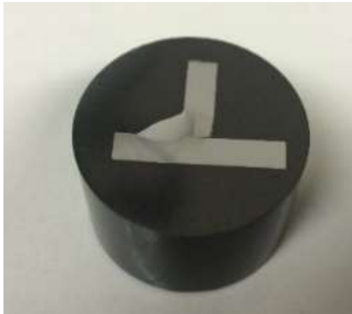
Figure 3-21 Example of mounted and polished sample
