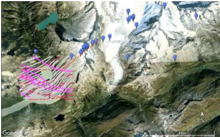
Figure 56: Plane fitting for a number of the located events presented as an orange dotted line. The plane agrees with the fractures reported by Schneeberger et al. (2017) and Stillings (2020).
