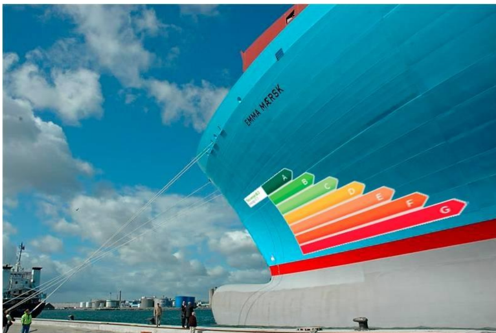
Figure 2.8: Rightship's GHG emissions rating scale depicted on the port bow of the M/V Emma Maersk (Rightship, 2013b)
