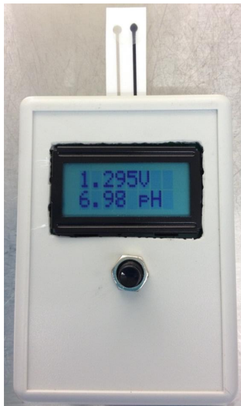
Figure 18: This shows a typical pH measurement. The disposable sensor is attached to the measurement device on the top. After calibration the integrated monitor shows the measured voltage and the corresponding pH of the applied sample.
