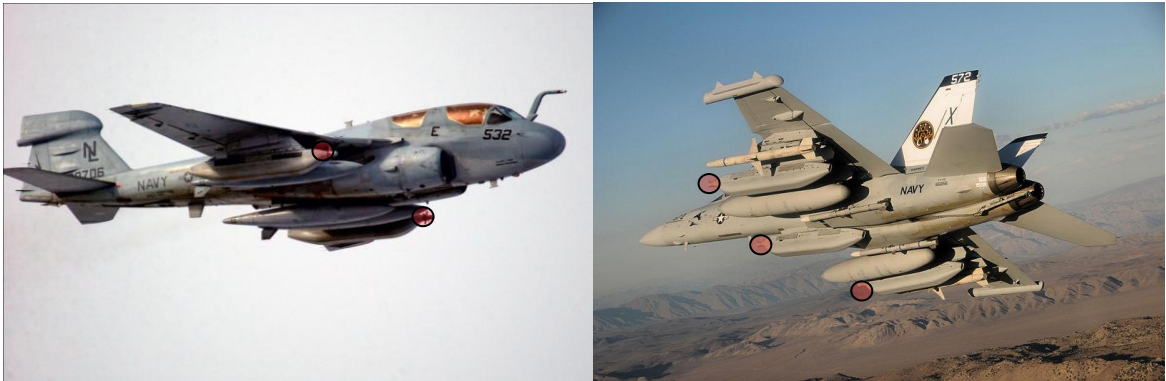
Figure 39- Pod mounted RATG for ALQ 99 on EA 6B [77] and F18G [78]
