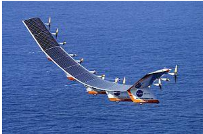
Figure 31- Illustration of Helios solar UAV [63]
