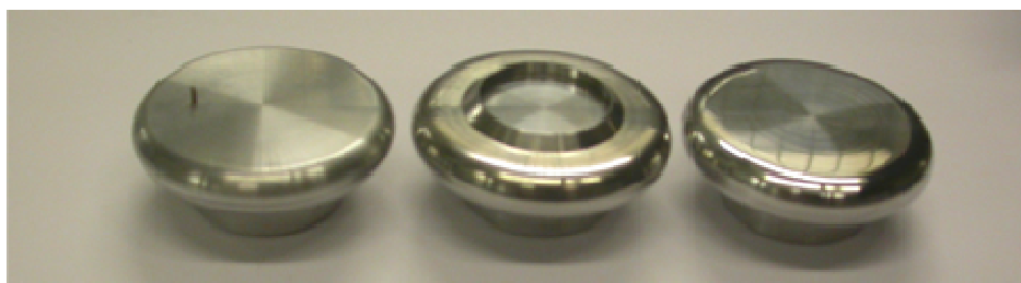
Figure 3.5. Photograph of different high-voltage electrodes. From left to right: type A, type B and type C.
