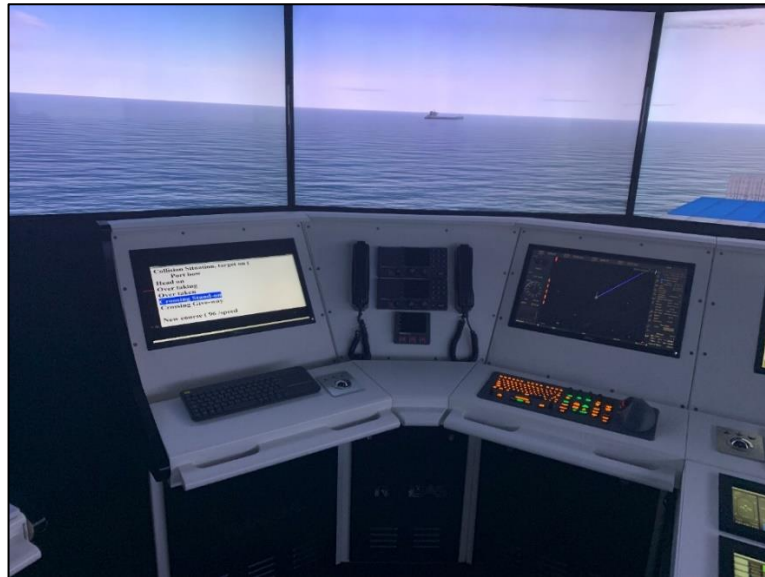
Figure 77 The Automatic Collision Avoidance instruction screen on the bridge simulator
