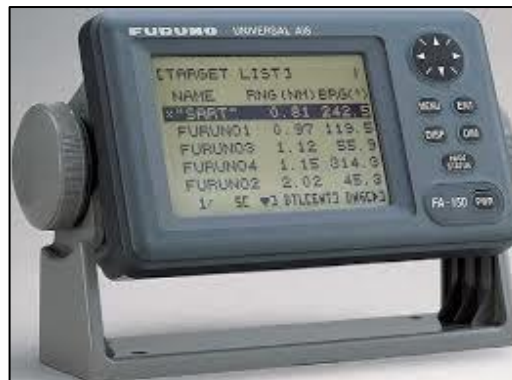
Figure 22 Furuno AIS system (ThitonikMarine, 2019)
