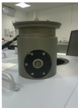
Figure 2.8 The sample cell removed from the FTS showing one of the circular windows that allow the infrared beam to pass through the cell
