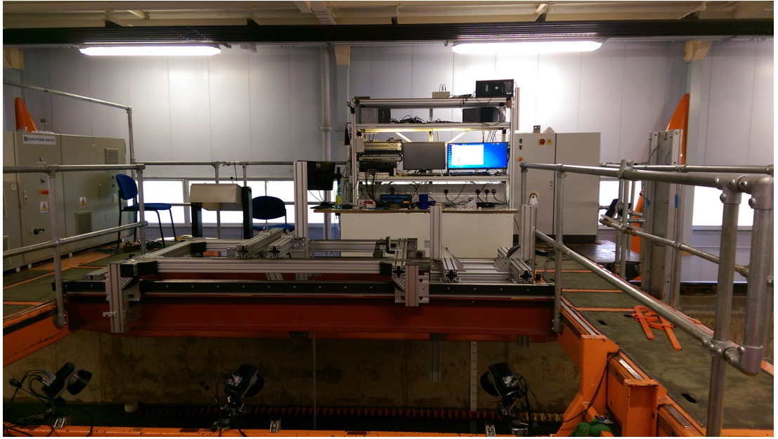
Figure 3.4: Qualisys system: three tracking cameras out of five plus recording PC
