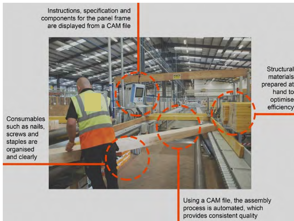
Figure 55. Framing station (semi-automated production) with annotated highlights.
