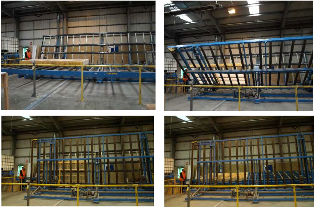
Figure 61. Example of a butterfly table, which rotates the panel from horizontal to vertical on one steel frame ‘wing’, the timber panel is then transferred onto the opposite wing and rotated back to horizontal position, 180° flipped from its starting position.
