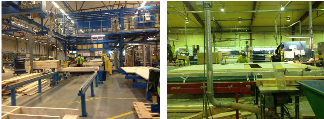
Figure 82. Closed timber panel production in Sweden: automated assembly line and manual benches. Author's own images. June 2017.
