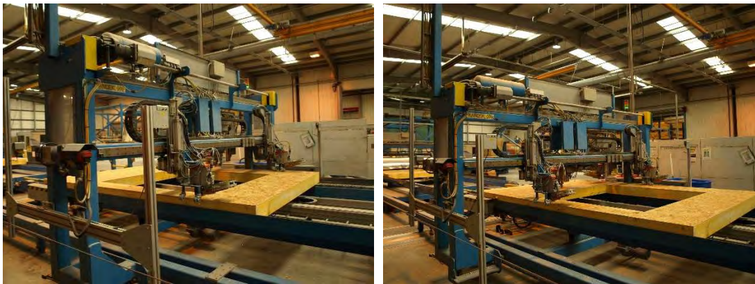
Figure 57. Nailing bridge example with 2 nail guns, which move along support beams on 3 axis and automatically nail the OSB sheet to the timber frame in seconds.
