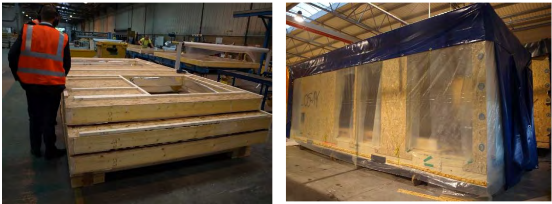
Figure 46. Examples of timber stud systems – closed panels (left) and volumetric (right).
