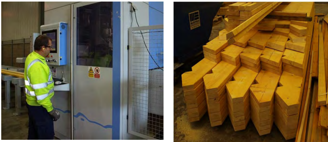
Figure 58. Example of a CNC saw, which cuts intricate shapes accurately and quickly and reduces the risks of working with sharp cutting tools.
