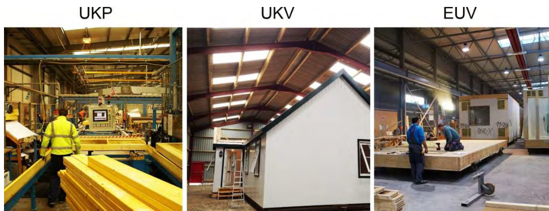
Figure 49. Examples of automated (UKP) and manual working environments (UKV, EUV).
