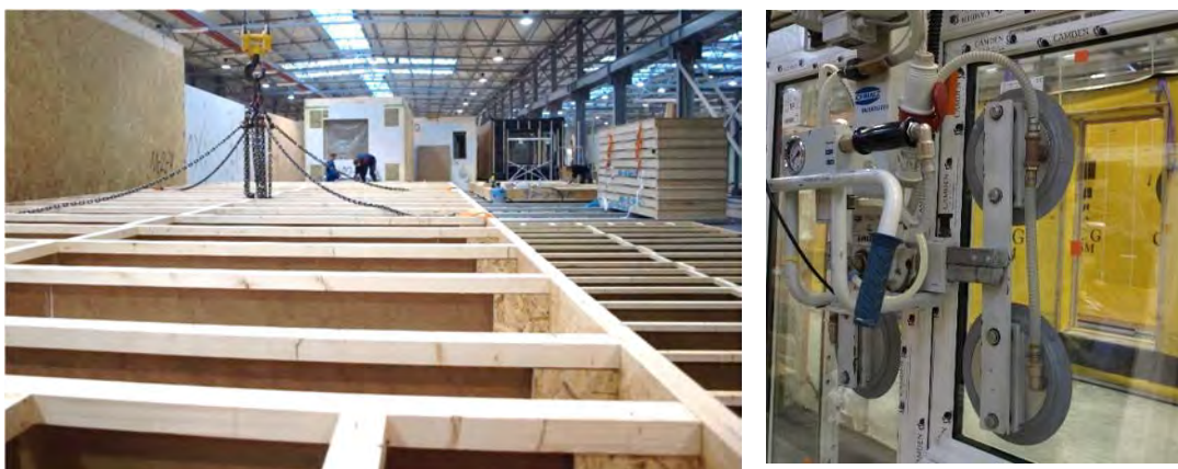
Figure 60. Example of an indoor crane, attached to a floor cassette and a vacuum machine.
