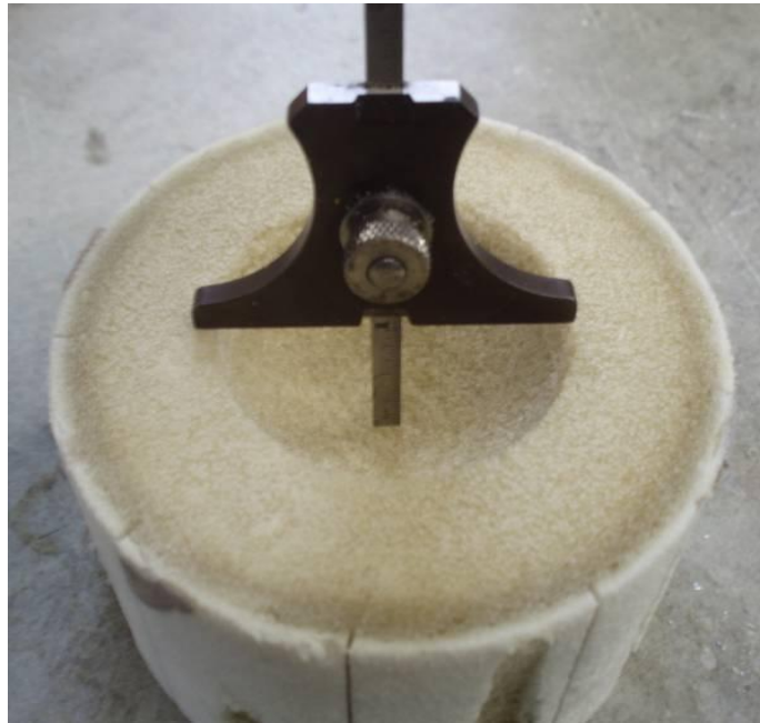
Figure 14: Illustration of the measurement of the depth of the reamed cavity to be tested, using a depth gauge.
