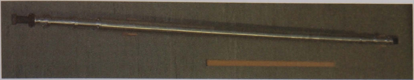
Figure 6-1 Aluminium helically corrugated waveguide including helical tapers, elliptically shaped polarisers and rectangular-to-circular converters with metre stick shown for perspective.
