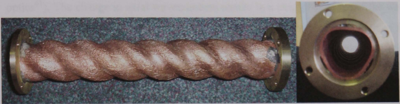
Figure 6-3 Digital photo's of the copper helically corrugated waveguide.
