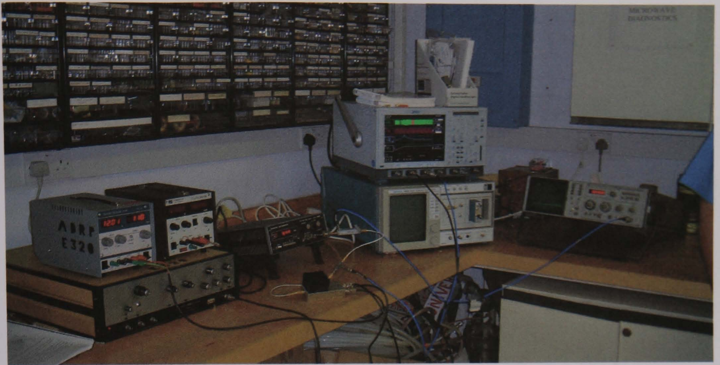
Figure 7-6 Experimental set-up showing from left to right, Systron Donner Pulsed generator swept voltage source, Thurlby power supply to drive microwave oscillator, solid-state microwave oscillator, Marconi local oscillator, mixer, fast digitising oscilloscope and spectrum analyser.
