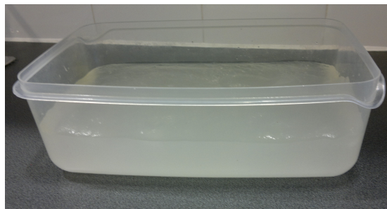
Figure 3.3B: Tissue Mimicking material made from wheat flour adhesive
