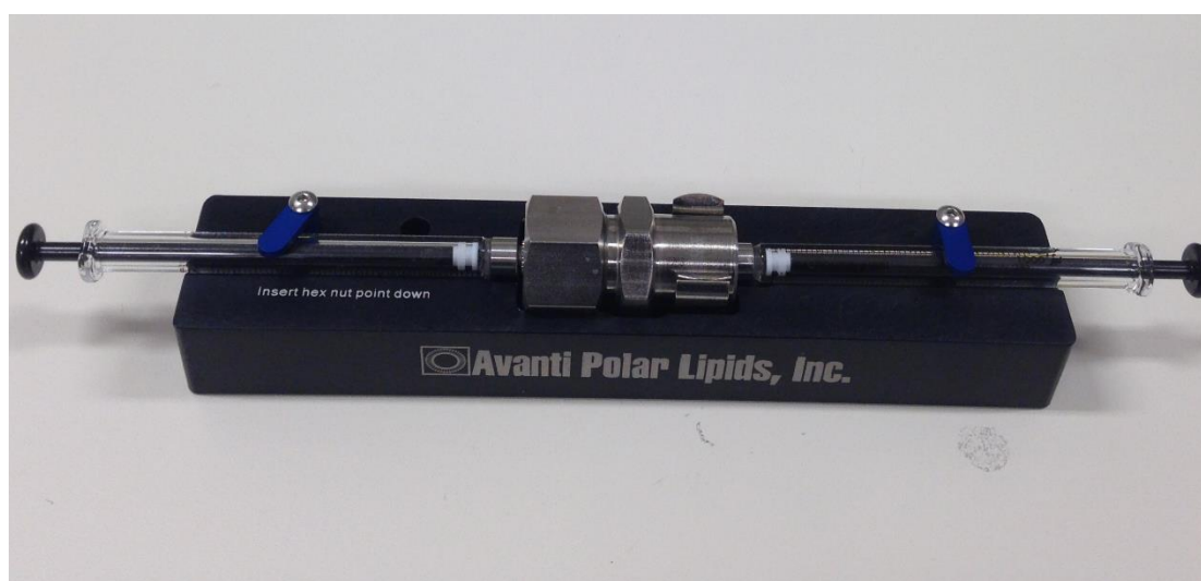
Figure 2.1 Avanti miniextruder containing a 100 nm pore diameter polycarbonate (PC) membrane used for particle size reduction.
