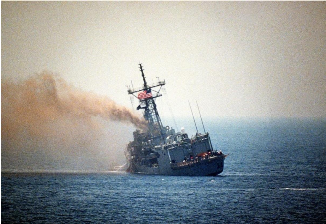
Figure 1.4. Heel after damage (Miller and Shattuck, 2004)
