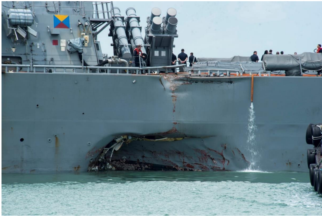
Figure 1.8. A large damaged opening causing flooding (Department of the Navy of USA, 2017)
