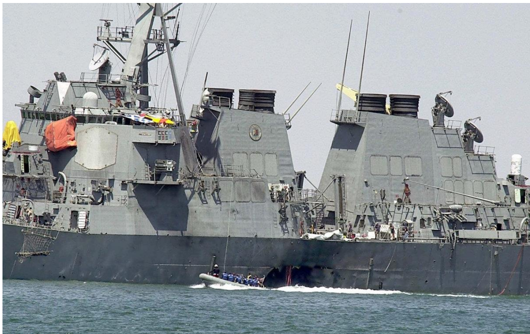
Figure 1.2. Damaged hole at waterline (Brown, 2004)
