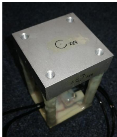
Figure 3.13. Torsional moment ( M_z ) marked on transducer
