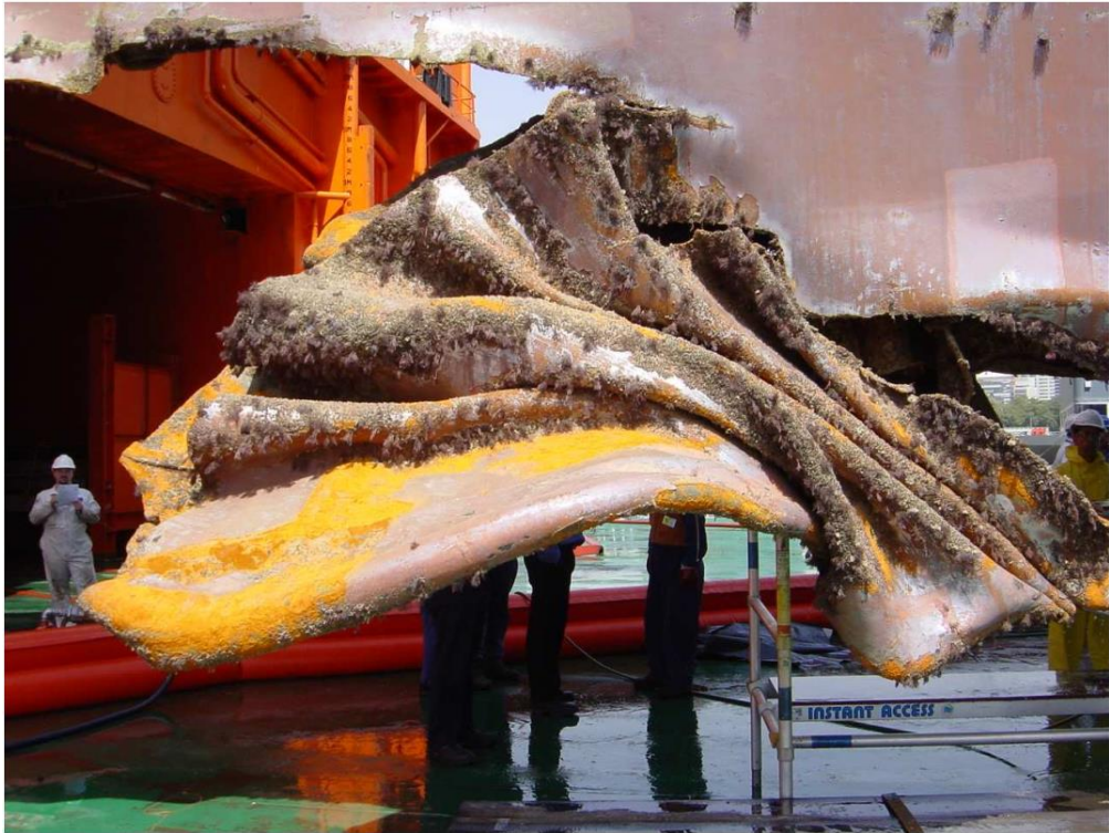
Figure 1.5. Tear damage (Bole, 2007)
