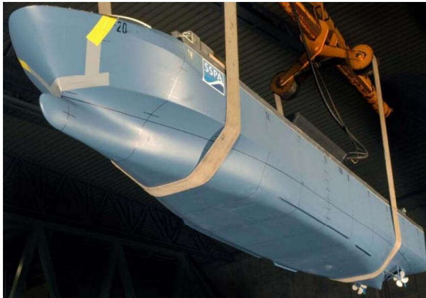
Figure 2.3. Physical Ro-Ro ship model for reconstruction of Estonia (note the visor attached at bow) (SSPA Consortium, 2008)
