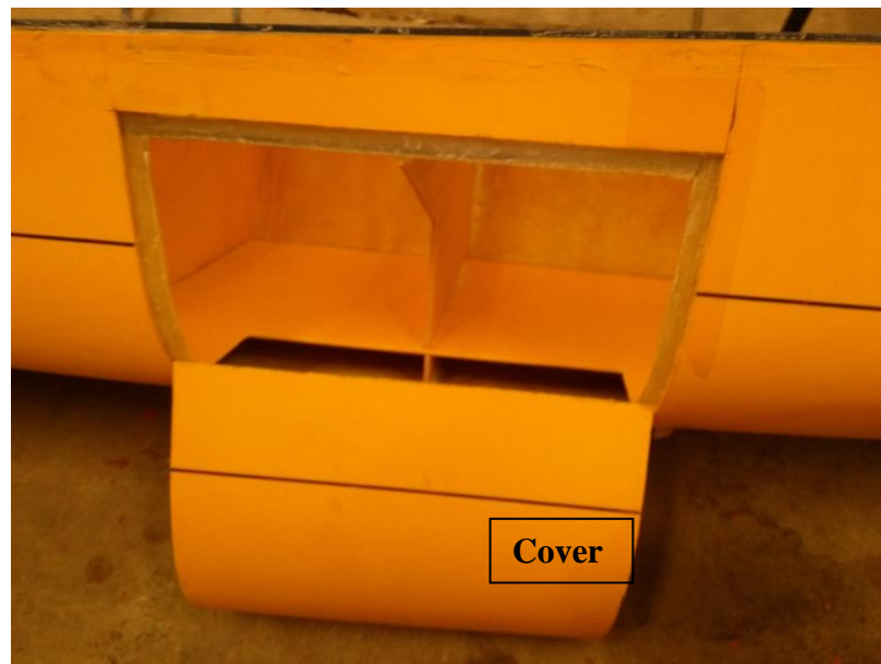
Figure 5.14. Damaged opening in physical model (Cover is unattached)
