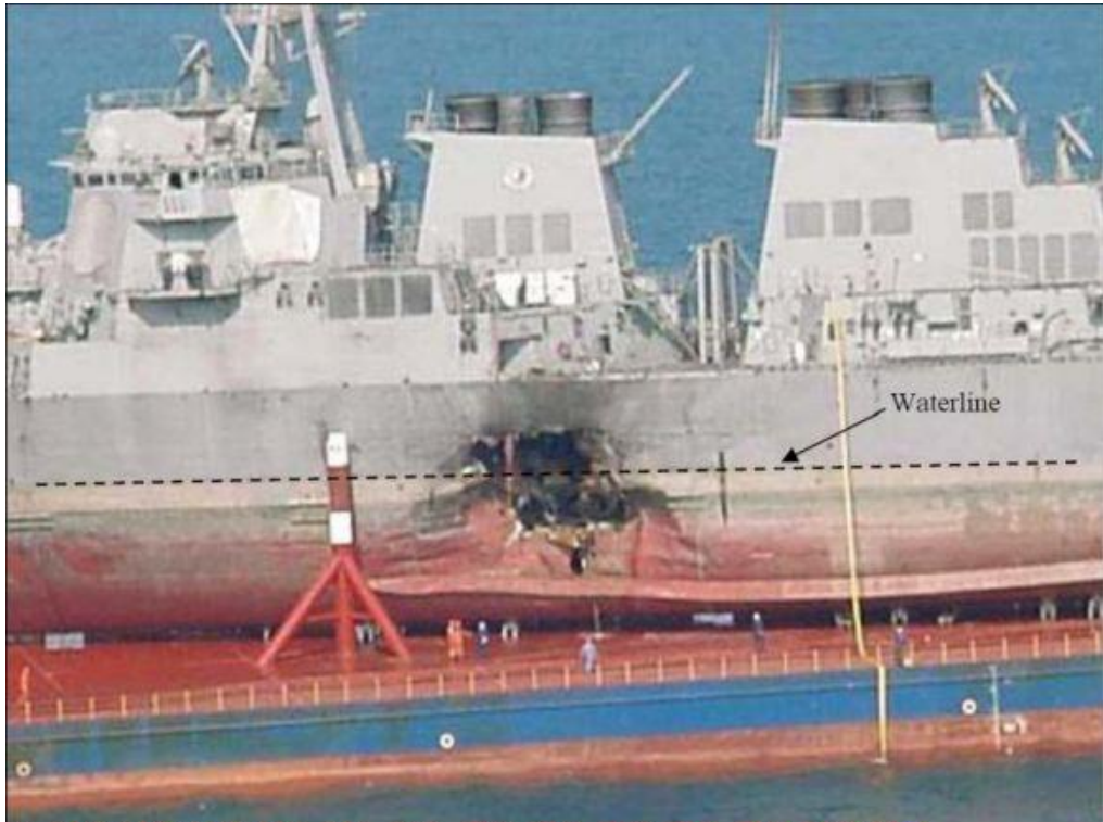
Figure 1.1 Damaged hole at waterline (Brown, 2004)
