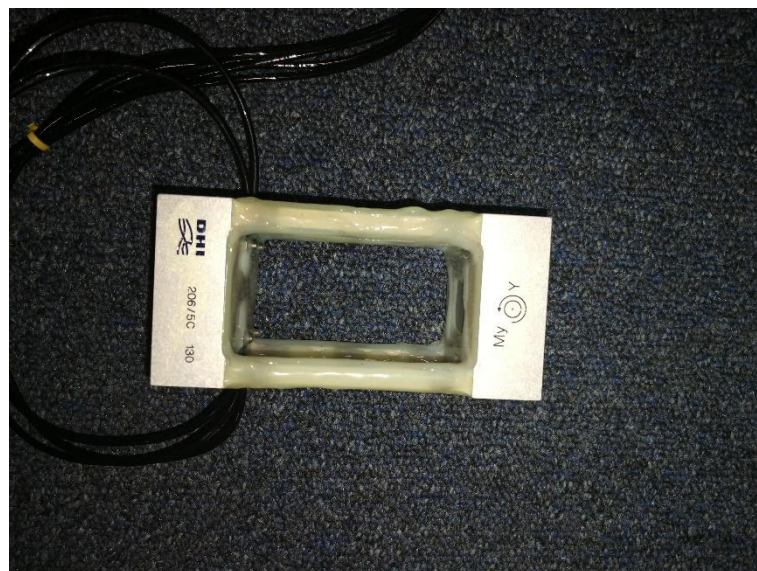
Figure 3.10. Type 206/5C 5-Component force gauge by DHI
