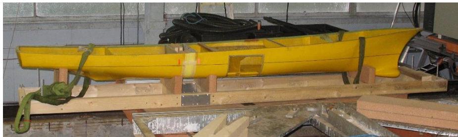
Figure 3.20. Wooden support used to hold the ship model
