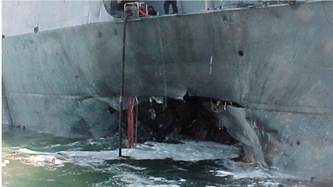
Figure 1.3. Water inflow from damaged opening (Brown, 2004)
