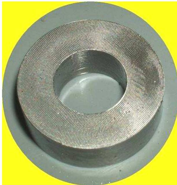
**Figure 4.8:** Photograph of ring specimen with textured surface
