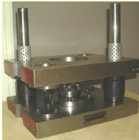
**Figure E.4:** Compression tool set with platens
