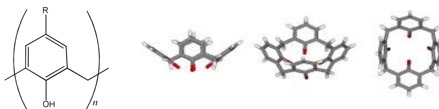
Figure 1.9 The general structure and three-dimensional structure of the calix[ n ]arenes, n = 4-20.
