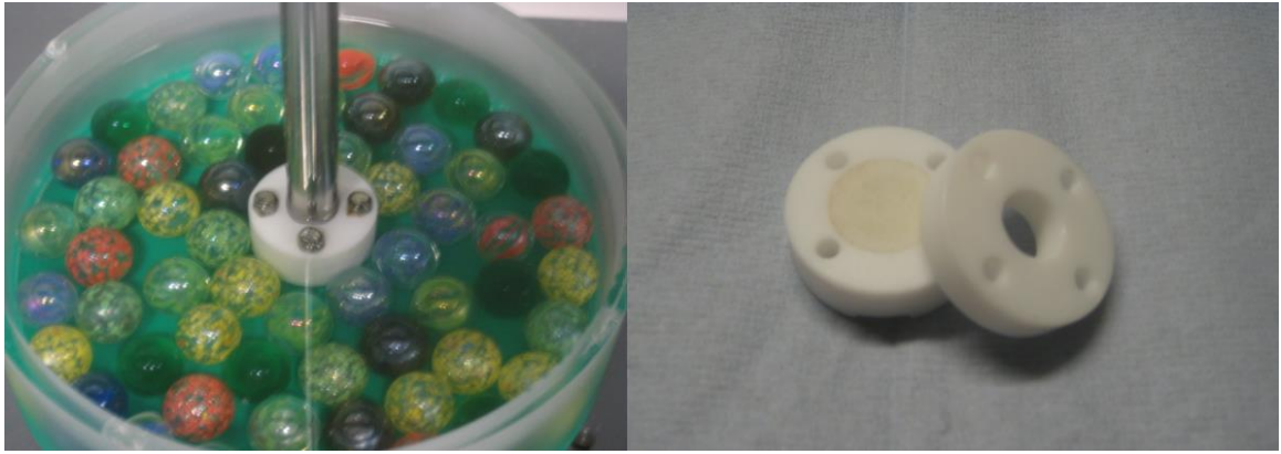
Figure 4-4. Picture of confined compression chamber used for cartilage testing; with water bath and indenter (left), and unassembled (right). The coloured marbles were used to reduce the volume of the external solution required to immerse the chamber.
