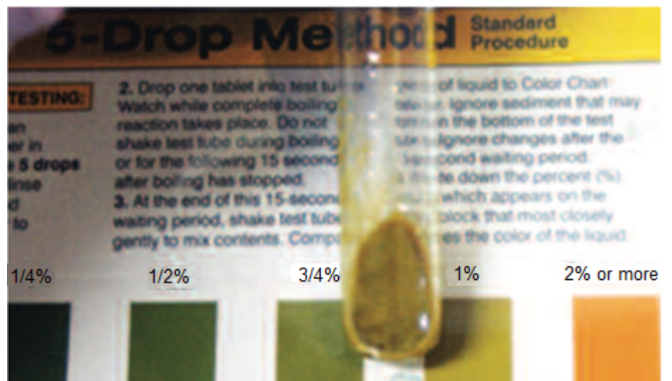
Figure 2.7 Colour chart to quantify the glucose using Clinistest® Reagent Tablet (adapted from Clarke and Foster, 2012)
