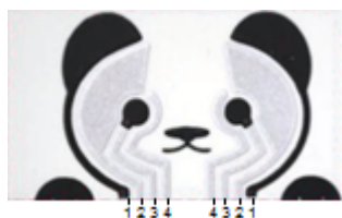
Figure 2.26 Panda-shaped screen-printed three electrode system with iontophoresis electrodes (adapted from Kim et al., 2018)
