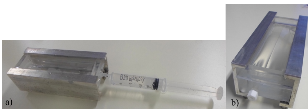
Figure 5.10 a) Diffusion cell with syringe to fill the buffer solution b) diffusion cell with closed holes using PTFE caps
