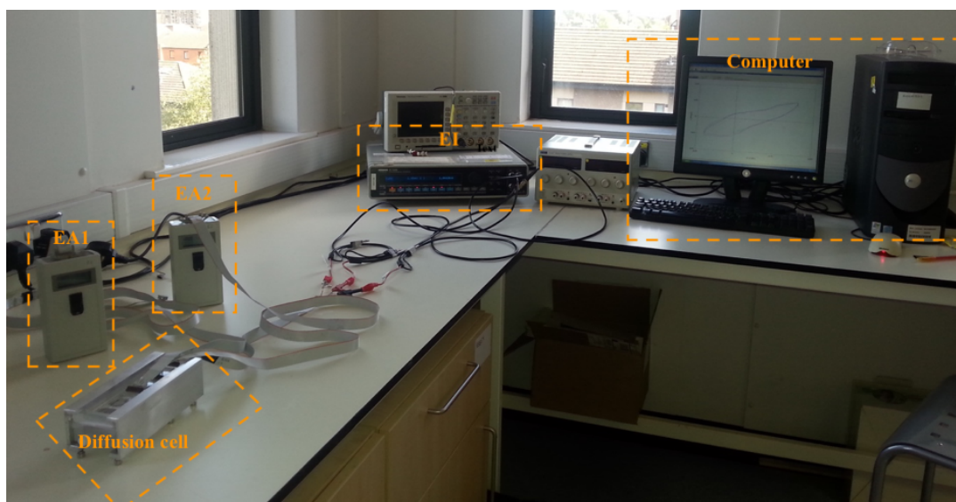
Figure 6.32 Measurement setup for RI experiments using glucose sensors with and without AC foam. E1 is connected to the computer and was used to perform CV to ensure sensor performance. EA 1 was responsible to apply the iontophoretic current between E1 and E2 electrodes and also to take CV from the E1 electrode. The EA2 took CV measurements from the E2 electrode and from the control electrode.
