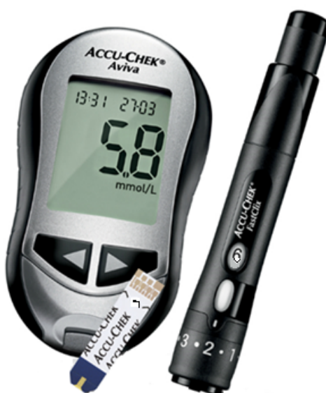
Figure 2.12 Example of a blood glucose meter with a test strip and a lancing device from Accu-Chek® Aviva (adapted from Healthcare4All, 2014)
