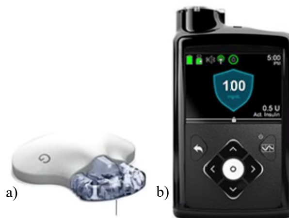
Figure 2.16 Medtronic's CGMS with a) Guardian 3 glucose sensor and Guardian 3 Link transmitter (adapted from Medtronic, 2019a) b) Minimed 670G pump (adapted from Medtronic, 2019b)
