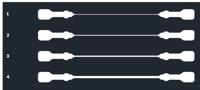
Figure 3.16: CAD drawing of a microfluidic mask showing geometries of microfluidic channels to be produced. The mask consists of 4 straight channels with varying widths, with sections for inlets and outlets to be punched.
