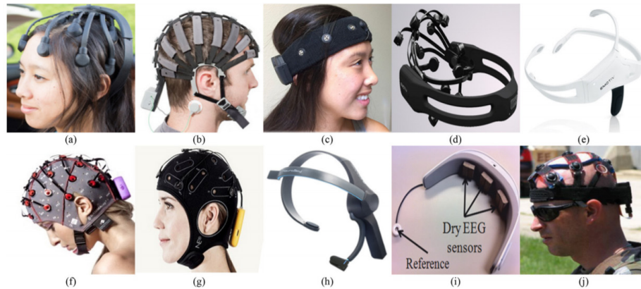
Figure 2.10. Different portable wireless EEG headsets. (a–c) Miniature dry-electrode wireless acquisition by Cognionics, (d and e) EPOC and Insight wireless EEG acquisition by Emotiv, (f) g.Nautilus wireless EEG acquisition by g.tec, (g) ENOBIO wireless EEG system by Neuroelectronics, (h) MindWave mobile EEG headset by NeuroSky, (i) wearable EEG headset, and (j) wireless EEG headset by Advanced Brain Monitoring. Adapted from (Minguillon et al., 2017; Chum et al., 2012).
