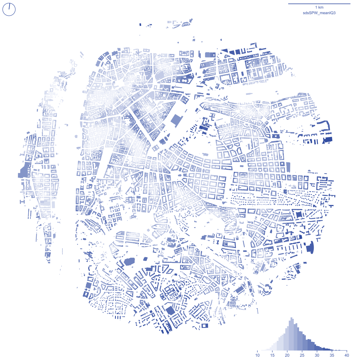
Figure 7.13: Spatial distribution of the interquartile mean of a width of a street profile measured within three topological steps on morphological tessellation in the area of Prague's city centre and its surroundings.
