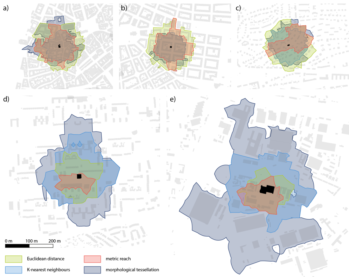
Figure 6.27: Comparison of boundaries of aggregations defined by each of the tested method for 4 topological steps and equivalents (200 metres, 70 neighbours). a) Old Town, b) Vinohrady, c) Hanspaulka, d) Jižní Město, e) Malešice
