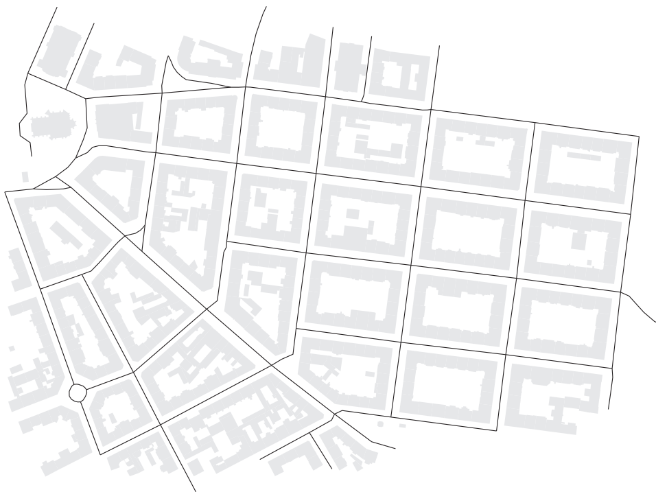
Figure 6.3: Illustration of street network represented as street centrelines, from which can be derived both street edge and node.
