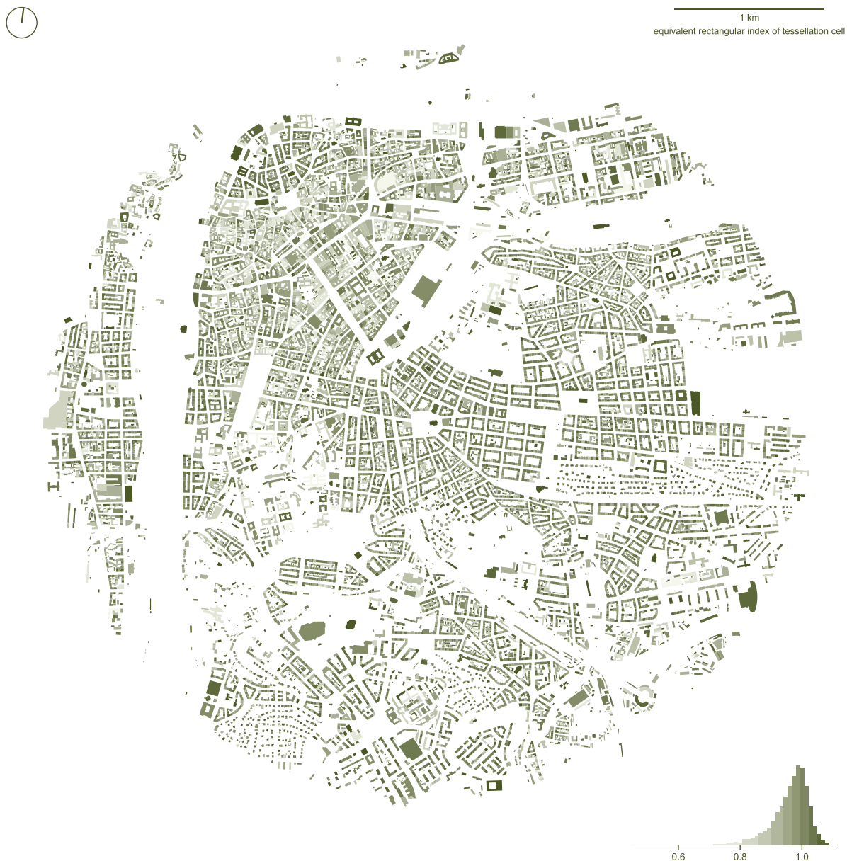
Figure 7.4: Spatial distribution of equivalent rectangular index of tessellation cell in the area of Prague's city centre and its surroundings. Figure illustrates visually unclear spatial patterns.
