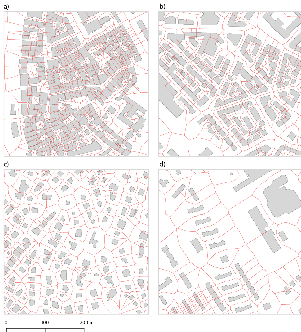
Figure 6.22: Morphological tessellation cells as generated across four different areas of Zurich; 4a) organic tissue of Niederdorf; 4b) compact tissue of Langstrasse; 4c) detached villas of Hottingen; 4d) mixed post-war development of Friesenberg.
