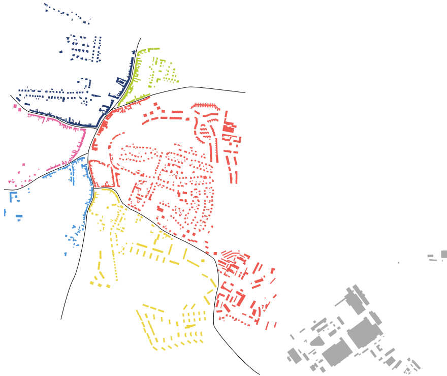
Figure 3.4: Illustration of sanctuary areas in a town Milevsko, Czechia. Main streets forming boundaries of SAs are marked as black lines. It is clear that SAs are composed of multiple heterogeneous patterns and do not function as a unit of urban form which would be sensible to use as OTU.
