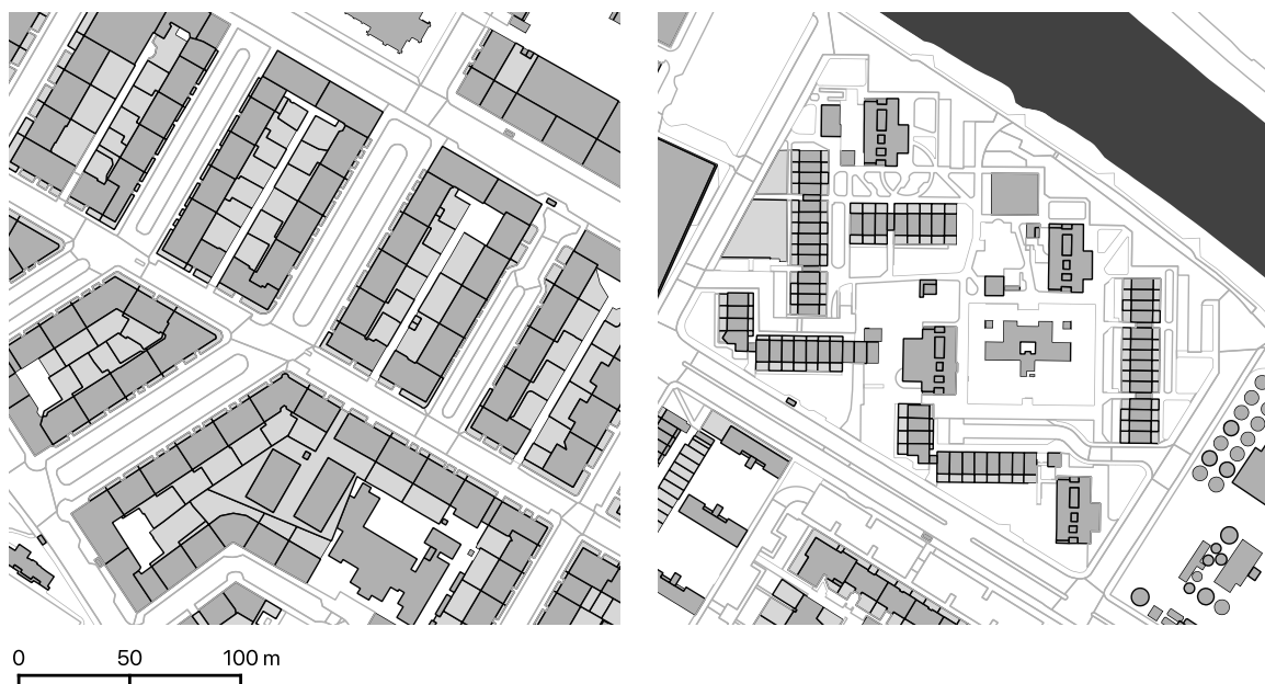
Figure 6.4: Comparison of traditional (left) and modernist (right) urban tissues in Glasgow. Plots are clearly better identifiable—even just visually—in the former, where distinction of public and private space is clear-cut, than in a modernist housing estate, where the transition between public and private is blurred. Source: Ordnance Survey MasterMap, January 2019 (EDINA Digimap Service)
