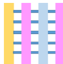
Parallel microchannels showing cell culture (yellow), hydrogel (blue) and media channels (pink)
