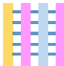
Parallel microchannels showing cell culture (yellow), hydrogel (blue) and media channels (pink)
