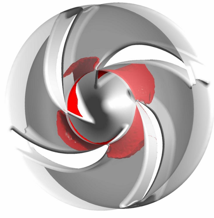
Figure 6.16 – Iso-surface of Water Vapour = 0.25 at NPSH_A = 5.7 m
