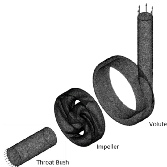
Figure C12 – Centrifugal Pump Case Study
