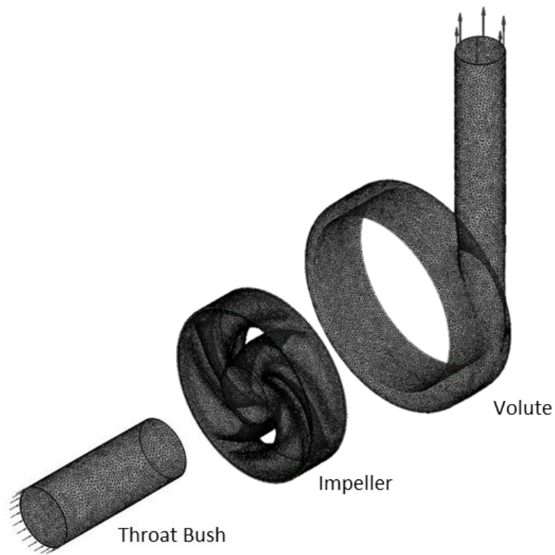
Figure 4.6 - Overall Case Mesh Construction
