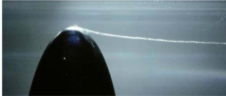
Figure 2.5 - Vortex Cavitation Generated by a Three-Dimensional Hydrofoil [5]
