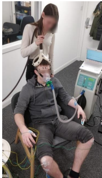
Figure.5.3. Experimental set-up where the participant is given IHT. Please note the grey reflective markers on the participant's forehead and on the double-cone coil. These clusters of markers are detected by motion capture cameras as objects and are used to aid the experimenter with coil placement.
