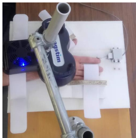
Figure.6.3. This figure shows the placement of the hand on the testing rig where the hand is trapped in place and the experimental rig that holds the weight of the cooling coil.
