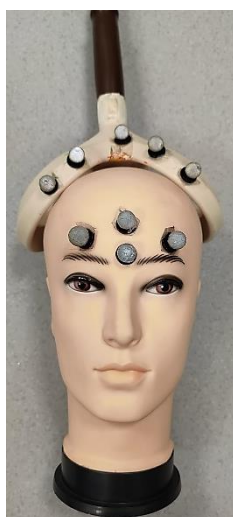
Figure.4.2. Positioning of the markers on the forehead and double- cone coil.
