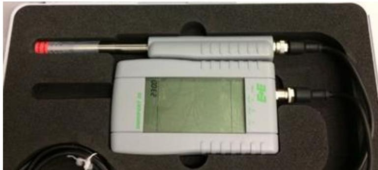
**Figure 3-3;** Omiport 20 oil humidity and temperature probe used to measure relative humidity of the dielectric fluids
