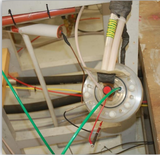
Figure 4.24: Photograph of the spark gap, used as a closing switch in the double Blumlein circuit, in the experiment.
