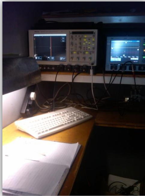
Figure 4.30: Screened room containing deep memory oscilloscopes, where microwave measurements were taken.
