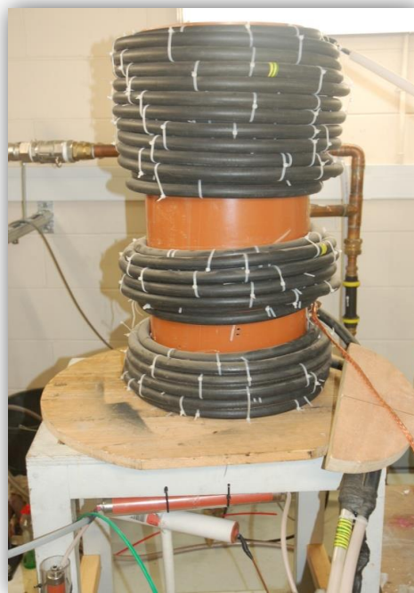
Figure 4.11: Experiment's inverting double Blumlein pulse generator.
