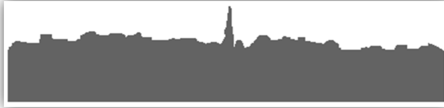
Figure 3.8: Illustration of the form of whiskers on the surface of stainless steel cathodes after exposure to fields of around 200kV/cm.
