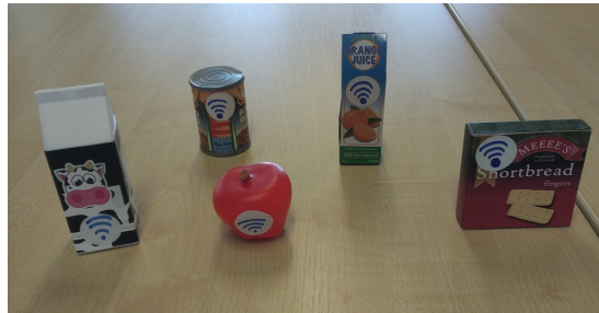
Figure 7.8: Some plastic food toys with the RFID tags attached to them. The white circle stickers with the WiFi-like symbol are the RFID tags.
