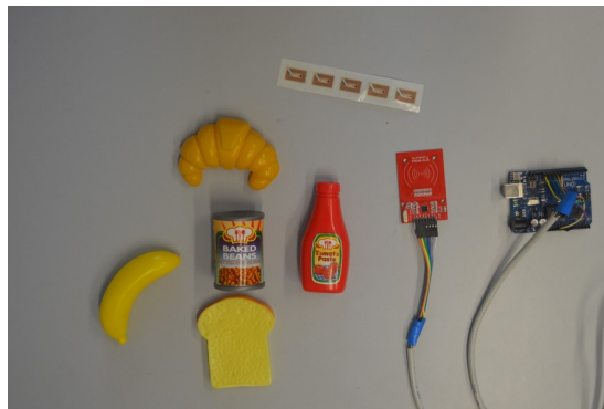
Figure 7.7: Initial food toys, RFID tags (a strip with small orange squares on the top of the image) and the Arduino microcontroller and the RFID sensor (red wired square next to the Arduino) used when the sensing technique was developed.
