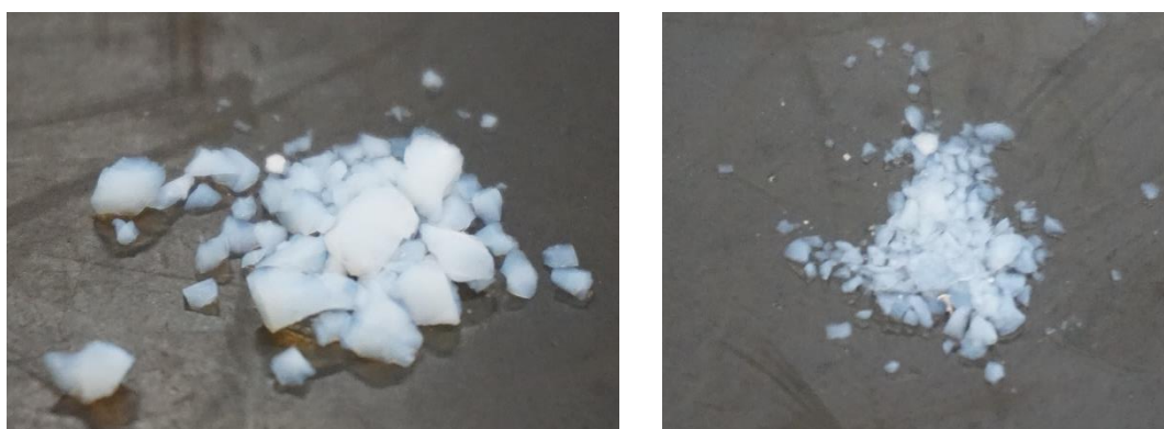
Figure 3-1 3500 \mu\text{m} (left) and 100 \mu\text{m} (right) silica aerogel particles used in this study.
