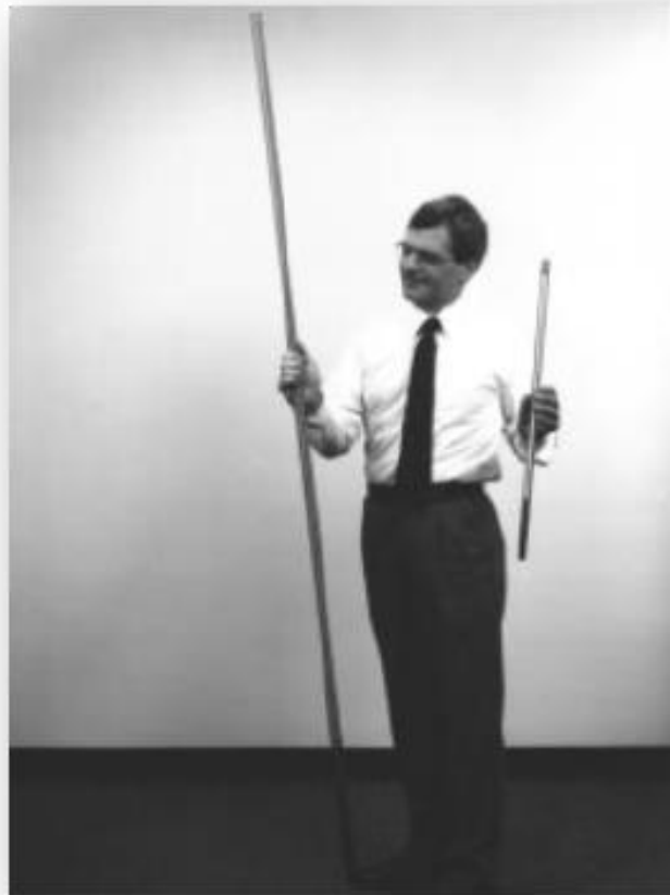
Figure 7; Illustration of the increased length of the Westinghouse single cell tube. Source DOE Report: George, R., 'Westinghouse Program Overview', in DOE Review Meeting (Morgantown, West Virginia US: Department of Energy, 1996), p.8.
