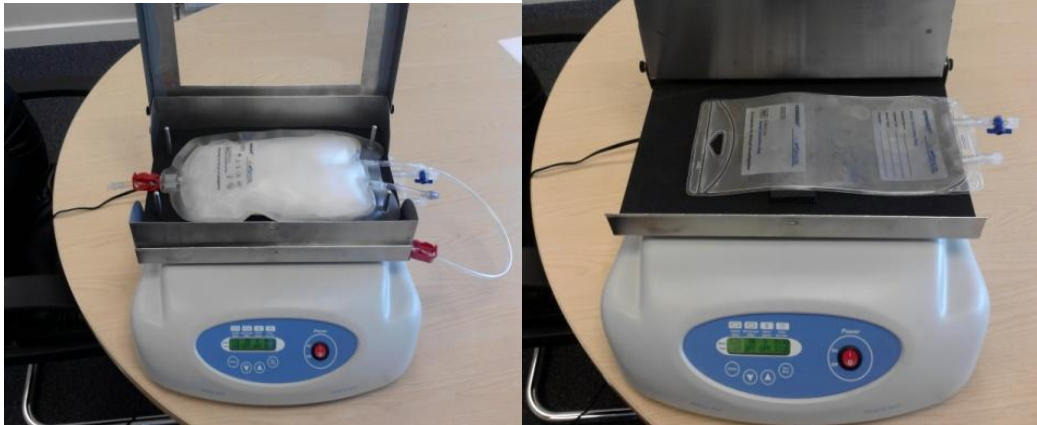
Figure 4.1 The HeoSep technology consists of 3 main components,1.theHemoSep bag2. The Fixed Rate Orbital Shaker and 3.The Transfer bag.
