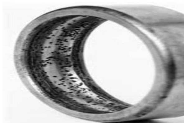
Figure 2.11: Corrosion on a tapered roller race [40].
